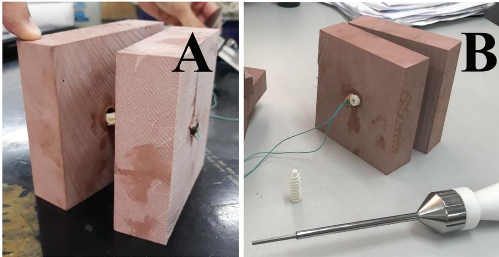
**Fig. 2** The samples. A - (Group 1) control group: the graft was fixed at the extremities of the polyurethane blocks with 30 mm-long and 9 mm-wide metallic interference screws, made of ASTM F136 titanium alloy (Traumédica); B - (Group 2) PLA group: the graft was fixed at the extremities of the polyurethane blocks with 30 mm-long and 9 mm-wide 3D-printed screws.
