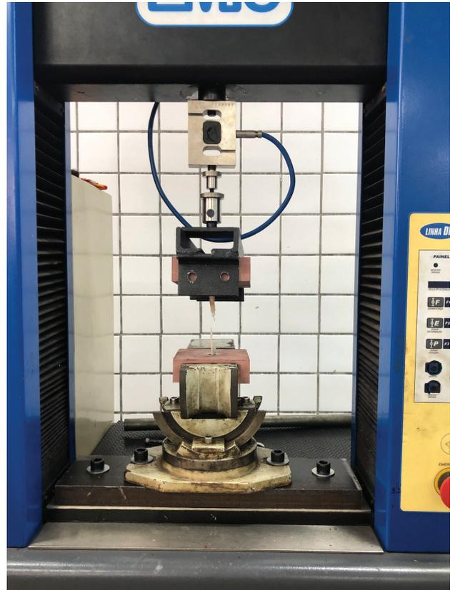
**Fig. 4** The sample (screw – block – graft – block – screw) on the testing machine (EMIC DL 10000 electromechanical universal testing machine).
