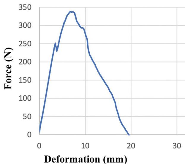
**Fig. 5** Graph of the Force (N)/deformation (mm) ratio suffered by the sample number 1 fixed with the PLA screw.
