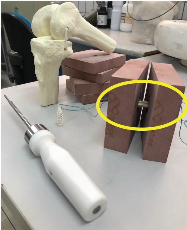
**Fig. 3** Test specimens displayed the following configuration (yellow circle): screw – block – graft – block – screw.
