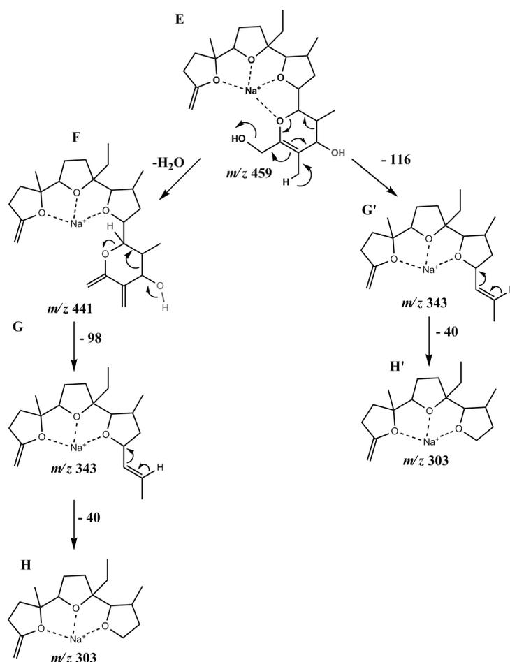
**Scheme 2.** The proposed fragmentation route showing the formation of product ion  $m/z$  303 in the positive ion ESI-MS/MS of the hydroxylated metabolite of monensin A - a crucial ion for the location of the site of hydroxylation.
