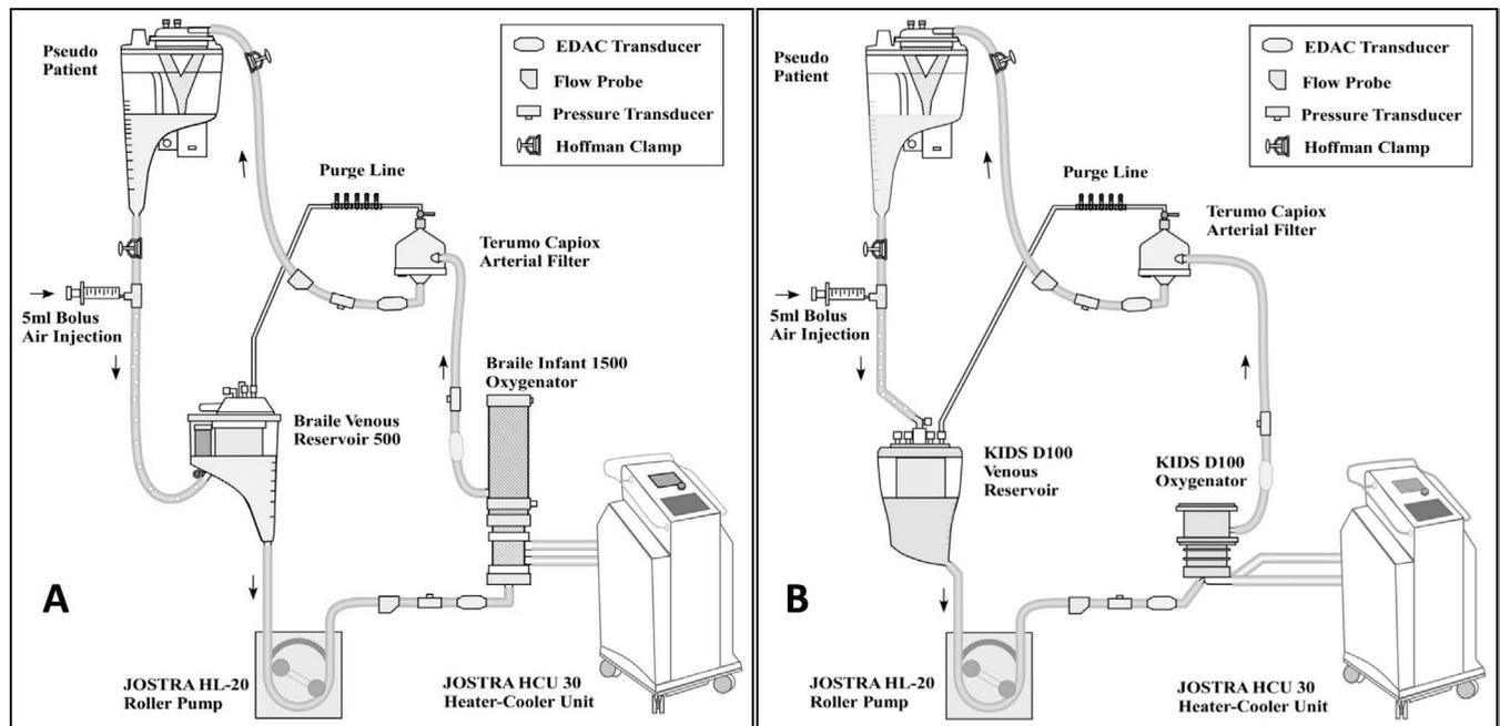
**Fig. 1** - Outline of CPB circuits with the Braille Infant 1500 oxygenator (A) and KIDS D100 oxygenator (B). (In the experimental set-up, the venous reservoir was placed directly on top of the oxygenator. They are separated in this schematic in order to display all components of the circuit clearly).
