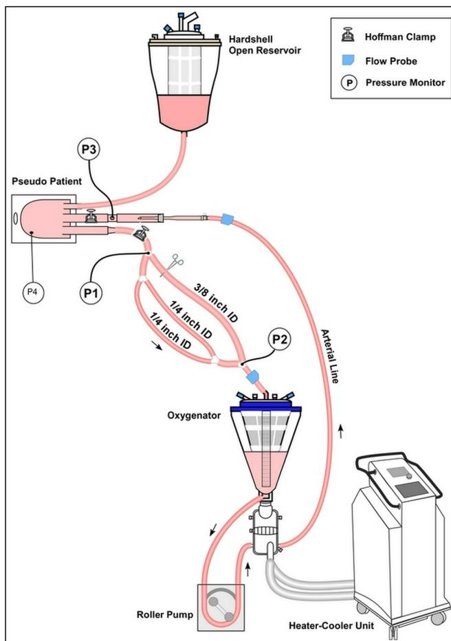
**Fig. 2** - Setup III for testing Circuits C and D using a soft bag as pseudopatient. During this experiment, venous pressure was kept at a constant range of 3 to 4 mmHg, simulating a controlled venous pressure more similar to a clinical scenario. Heater-cooler units allowed for experiments to be done at 35°C and 28°C. Hoffman clamp on the circuit arterial limb allowed for a constant post-cannula pressure of 50 mmHg.
