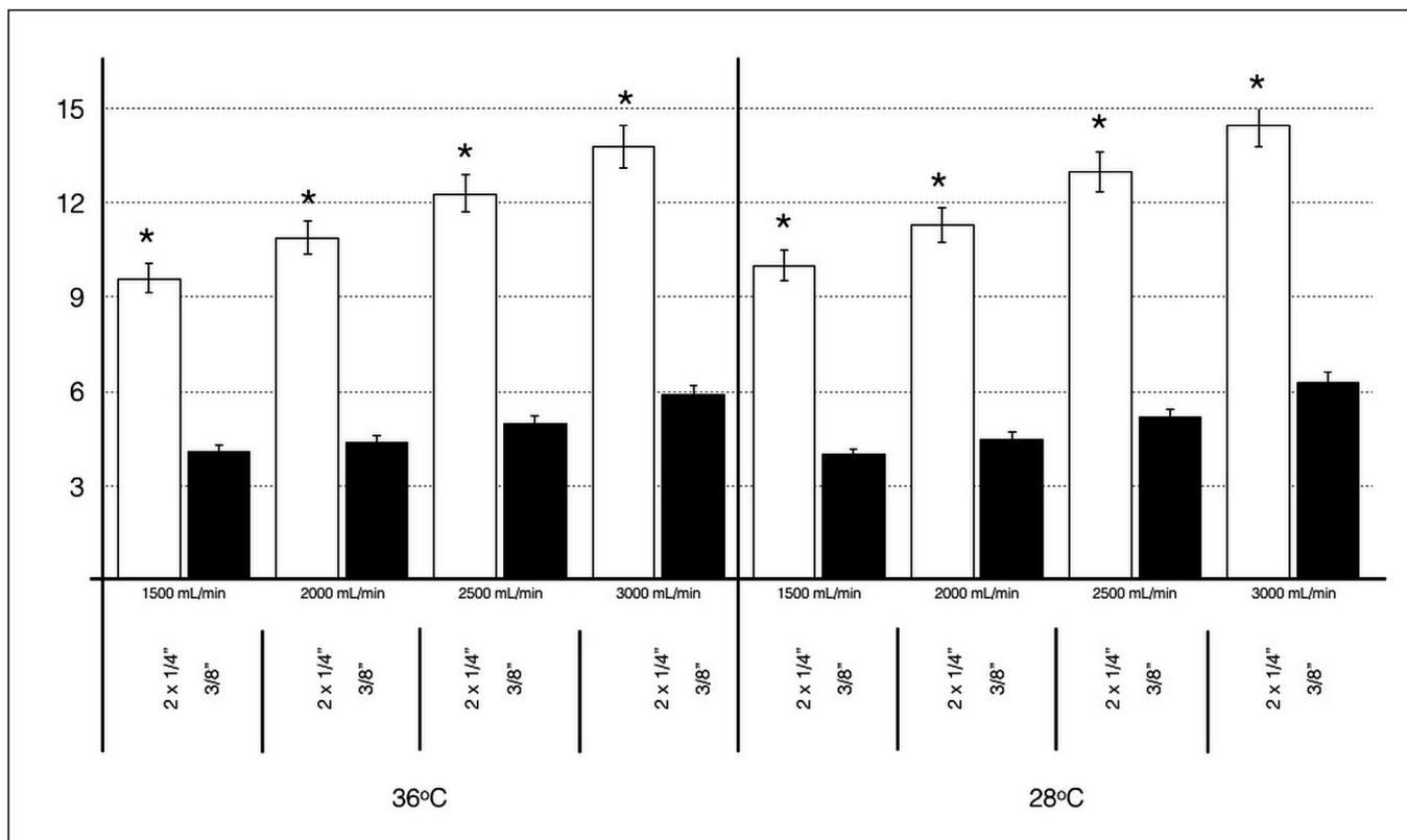
**Fig. 4** - Venous line resistance according to the arterial flow rate observed in Circuits C and D, in both normothermia and hypothermia (setup I), showing significant difference between them (\* $P < 0.001$ ).
