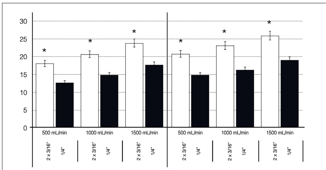
**Fig. 3** - Venous line resistance according to the arterial flow rate observed in Circuits A and B, in both normothermia and hypothermia (setup I), showing significant difference between them (\*P<0.001).
