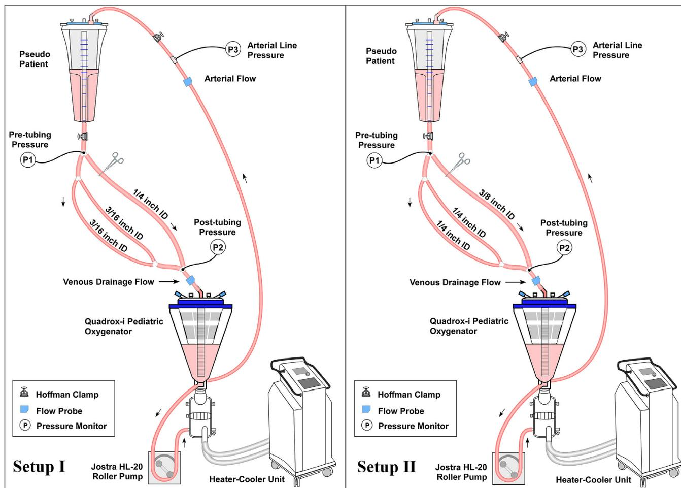
**Fig. 1** - Setup I allows for testing Circuits A and B. Setup II allows for testing Circuits C and D. Heater-cooler units allowed for experiments to be done at 35°C and 28°C. Hoffman clamp on the circuit arterial limb allowed for a constant post-cannula pressure.
