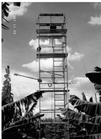
**Figure 4** - Eddy covariance tower installed within the study area of the banana orchard, located in Frutacor farm, Quixeré/Brazil.
