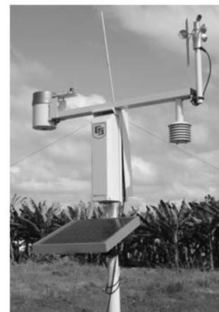
**Figure 3** - Automatic weather station (ET106) installed within the study area of the banana orchard, located in Frutacor farm, Quixeré/Brazil.
