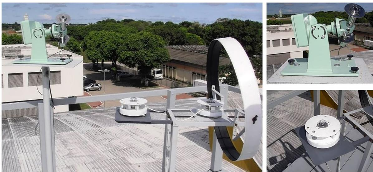
**Figure 2** - Solarimetric station: Kipp & Zonen CM5 pyranometer and pyrliometer assembled on the Eppley solar tracker.
