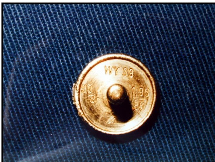
**FIGURE 4** – Photograph showing the Strontium-90 plate used to emit beta radiation.
