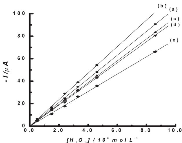
**Figure 3.** Analytical curves obtained for amperometric hydrogen peroxide detections with an Rh-PBMCPE at  $0.040\text{V}$ : (a) 1<sup>st</sup>, (b) 2<sup>nd</sup>, (c) 3<sup>rd</sup>, (d) 4<sup>th</sup> and (e) 5<sup>th</sup> days. Each analytical curve represents an average of 6 consecutive amperometric analytical curves performed in the same day.
