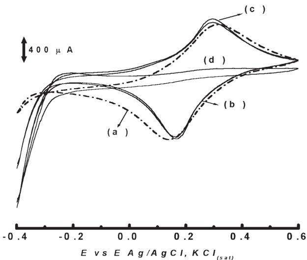
**Figure 1.** (a) 1<sup>st</sup>, (b) 30<sup>th</sup> and (c) 50<sup>th</sup> cyclic voltammograms carried out with a PB - carbon paste modified electrode (PB-CPME) and (d) with unmodified carbon paste electrode in a solution containing  $1.0 \times 10^{-3} \text{ mol L}^{-1} \text{ RhCl}_3$ ,  $0.5 \text{ mol L}^{-1} \text{ KCl}$  and  $0.01 \text{ mol L}^{-1} \text{ HCl}$  at  $60 \text{ mVs}^{-1}$ .
