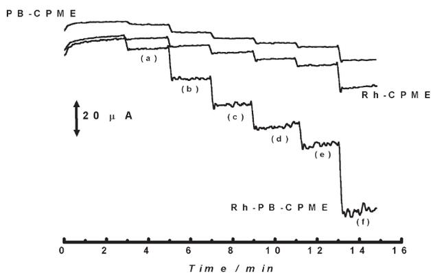
**Figure 2.** Amperograms recorded during the catalytic reduction of: (a)  $5.0 \times 10^{-6}$ , (b)  $1.4 \times 10^{-4}$ , (c)  $2.3 \times 10^{-4}$ , (d)  $3.2 \times 10^{-4}$ , (e)  $4.0 \times 10^{-4}$  and (f)  $8.6 \times 10^{-4} \text{ mol L}^{-1}$  hydrogen peroxide. Applied potential =  $0.040 \text{ V vs Ag/AgCl}$ . Supporting electrolyte = citric acid / sodium citrate buffer solution (pH 6.1) in  $0.5 \text{ mol L}^{-1} \text{ KCl}$ .
