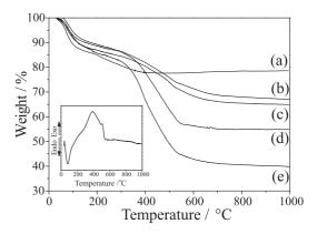
**Figure 1.** Termogravimetric curves, obtained in air atmosphere at  $8 \,^{\circ}$ C min<sup>-1</sup>: (a) TiO<sub>2</sub>; (b) TiO<sub>2</sub>/PANI-2A; (c) TiO<sub>2</sub>/PANI-1A; (d) TiO<sub>2</sub>/PANI-2B; (e) TiO<sub>2</sub>/PANI-1B. The inset shows the DSC curve for TiSn/PANI-1A sample.
