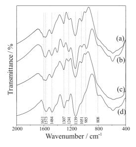
**Figure 2.** Infrared spectra: (a) TiO<sub>2</sub>/PANI-1A; (b) TiO<sub>2</sub>/PANI-1B; (c) TiO<sub>2</sub>/PANI-2A; (d) TiO<sub>2</sub>/PANI-2B.
