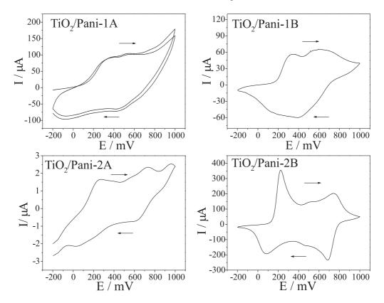
Figure 6. Cyclic voltammograms of the hybrid samples. Scan rate = 50 mV s<sup>-1</sup>; electrolyte = HCl/NaCl 1.0 mol L<sup>-1</sup> aqueous solution; reference electrode = Ag/AgCl.
