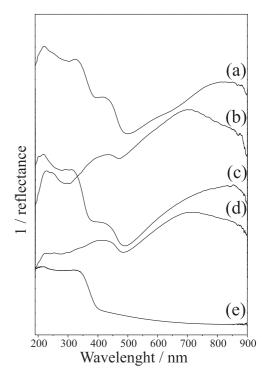
**Figure 4.** Reflectance UV-Vis spectra: (a) TiO<sub>2</sub>/PANI-1A; (b) TiO<sub>2</sub>/ PANI-1B; (c) TiO<sub>2</sub>/PANI-2A; (d) TiO<sub>2</sub>/PANI-2B; (e) TiO<sub>2</sub>.
