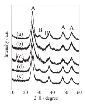
**Figure 5.** XRD pattern: (a) TiO<sub>2</sub>; (b) TiO<sub>2</sub>/PANI-1A; (c) TiO<sub>2</sub>/PANI-1B; (d) TiO<sub>2</sub>/PANI-2A; (e) TiO<sub>2</sub>/PANI-2B.
