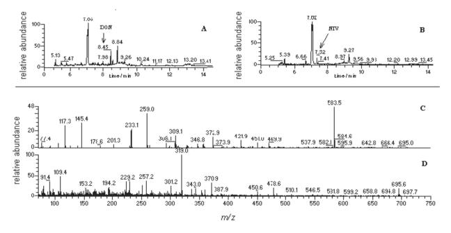
**Figure 2.** Chromatogram of tryfluoroacetyl derivatives of a corn sample contaminated with deoxynivalenol and nivalenol (A). Chromatogram rebuilt with most characteristics mass fragments for deoxynivalenol and nivalenol trifluoroacetyl derivatives (B). Mass spectrum of deoxynivalenol, trifluoroacetyl derivative (C). Mass spectra of nivalenol, trifluoroacetyl derivative (D). Chromatographic conditions in experimental.
