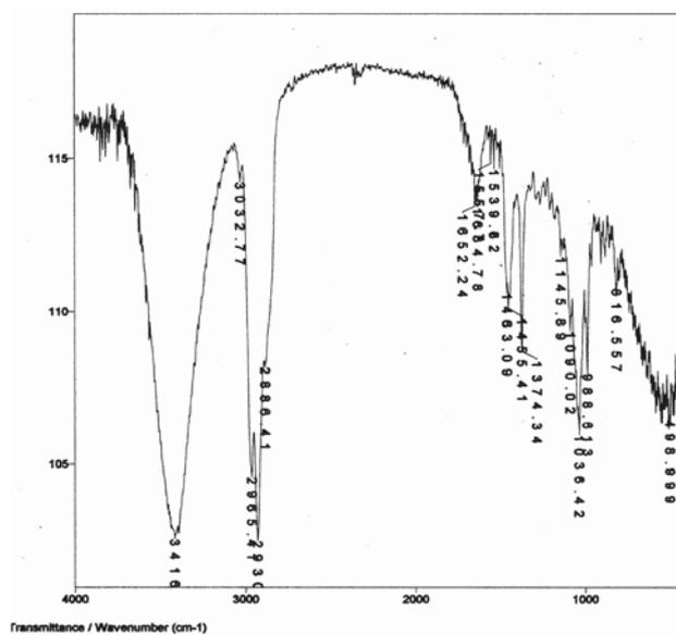
Figure S23. FTIR spectrum of compound 13.
