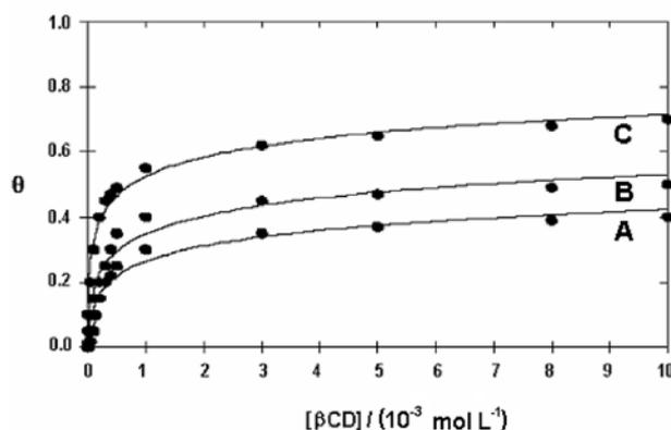
**Figure 4.** Adsorption isotherms of  $\beta$ CD from  $0.1 \text{ mol L}^{-1}$  KF at 298 K onto dendrimer-tethered ferrocene on the modified gold electrodes: (A) Au/SAM/PG2-Fc, (B) Au/SAM/PG3-Fc, and (C) Au/SAM/PG4-Fc. Experimental points derived from Figure 3 ( $\bullet$ ) were fitted to the Frumkin isotherm model, Equation 9 (—).
