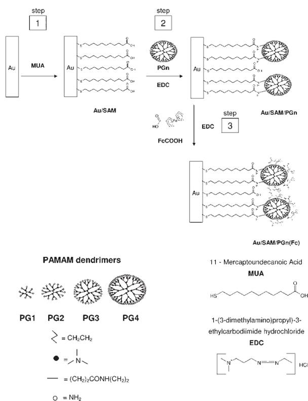
**Figure 1.** Schematic outline of the process used to prepare the gold electrodes compared in this study: (Step 1) Thiol modification of the gold surfaces to form Au/SAM; (Step 2) Dendrimer functionalization of the thiolated gold surfaces to produce Au/SAM/PGn, where n=1, 2, 3, 4; and (Step 3) Tethering of ferrocenyl moieties onto the immobilized dendrimers generating Au/SAM/PGn-Fc.
