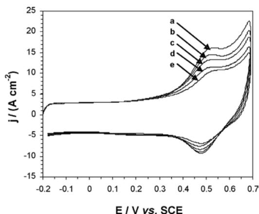
**Figure 3.** CV responses at  $dE/dt = 0.5 \text{ V s}^{-1}$  in  $0.1 \text{ mol L}^{-1}$  KF at 298 K at various concentrations of  $\beta$ CD for the modified electrodes Au/SAM/PG4-Fc after the introduction of (a) 0, (b) 0.001, (c) 0.1, (d) 0.5, and (e)  $1 \times 10^{-3} \text{ mol L}^{-1}$   $\beta$ CD. A similar trend was observed for the curves obtained for the systems Au/SAM/PG2-Fc and Au/SAM/PG3-Fc.
