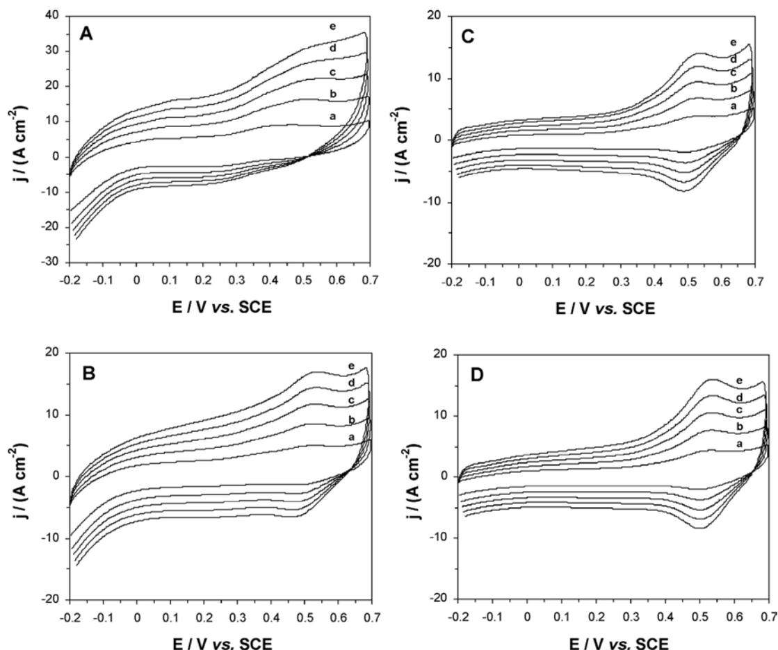
**Figure 2.** CV responses in aqueous  $0.1 \text{ mol L}^{-1}$  KF at 298 K of the four types of electrode: (A) Au/SAM/PG1-Fc, (B) Au/SAM/PG2-Fc, (C) Au/SAM/PG3-Fc, and (D) Au/SAM/PG4-Fc at (a) 0.1, (b) 0.2, (c) 0.3, (d) 0.4, and (e)  $0.5 \text{ V s}^{-1}$ .
