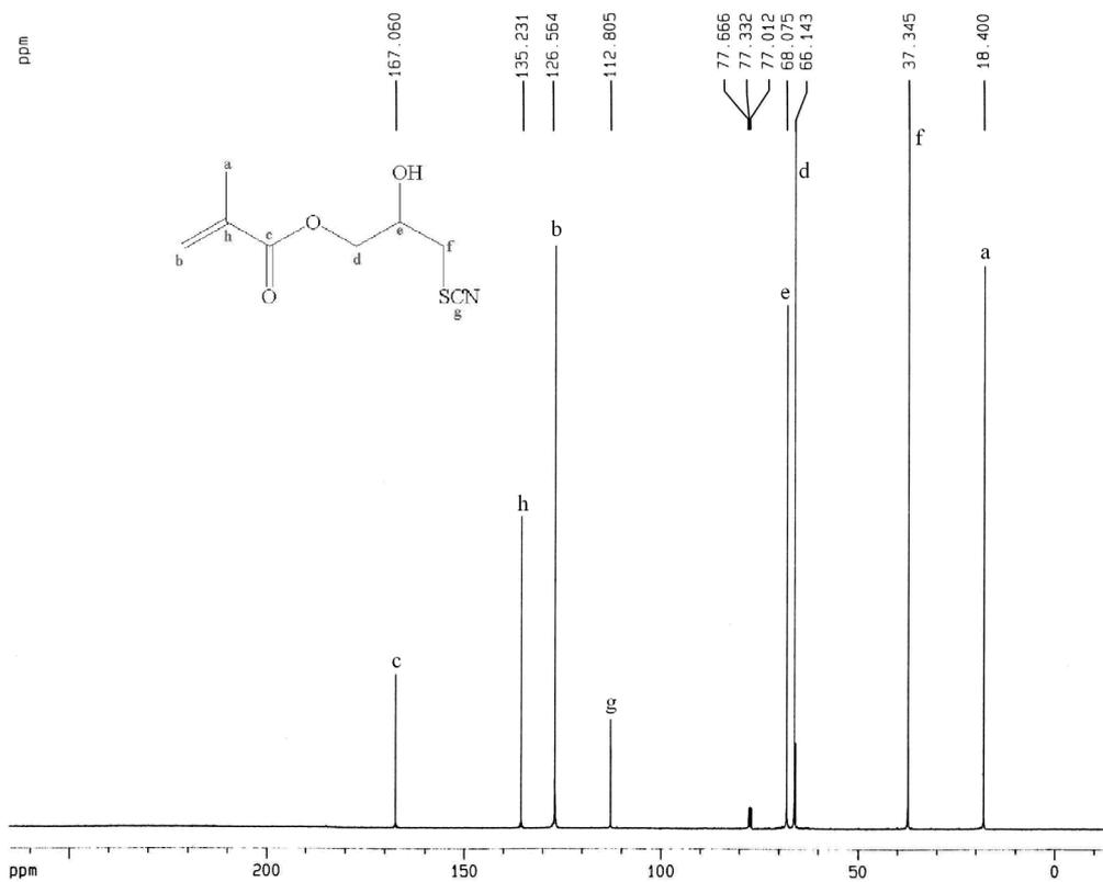
**Figure S3c.**  $^{13}\text{C}$  NMR of **6** (100 MHz,  $\text{CDCl}_3$ ).
