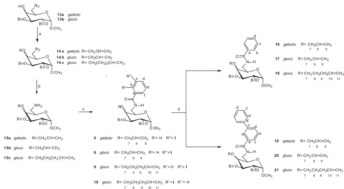
**Scheme 1.** Reagents and conditions: (a) Bu<sub>4</sub>NBr, 50% m/v aqueous NaOH, CH<sub>2</sub>Cl<sub>2</sub> or ethyl ether, allyl bromide or 5-bromo-1-pentene, rt; (b) LiAlH<sub>4</sub>, THF, rt; (c) 3- or 2-iodobenzoyl chloride (2 equivalents), 10% m/v aqueous NaOH, CH<sub>2</sub>Cl<sub>2</sub>, ice bath; (d) Bu<sub>3</sub>SnH (1.5 equivalents), AIBN (catalytic amount), benzene, N<sub>2</sub>, reflux.
