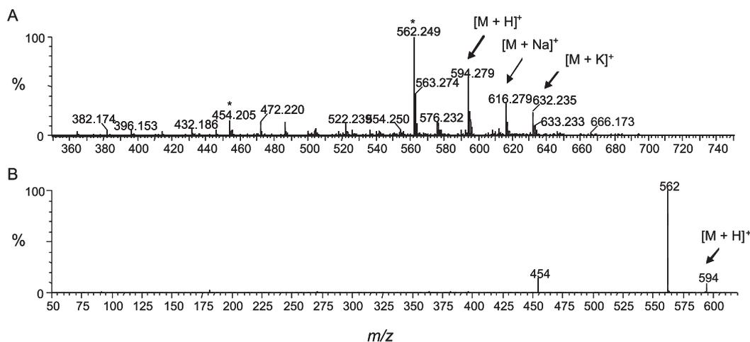
**Figure 3.** A: ESI-MS of product **19**; B: ESI-MS/MS of the protonated molecules of **19**. Ions marked by an asterisk are fragments due to  $\text{CH}_3\text{OH}$  and  $\text{PhCH}_2\text{OH}$  loss that arise likely from in-source collision-induced dissociation.
