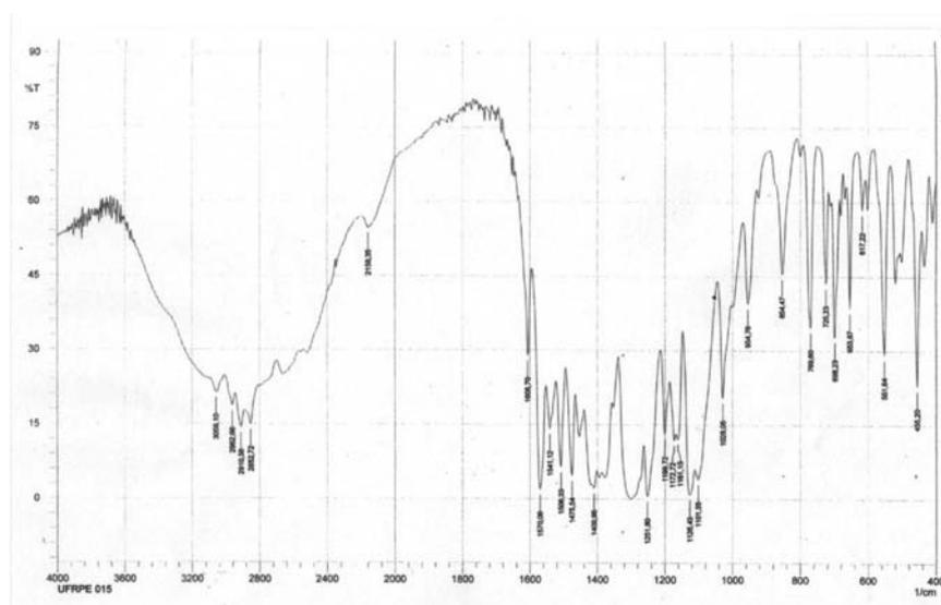
Figure S7. Infrared spectrum (KBr, cm<sup>-1</sup>) of 2a.
