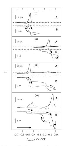
**Figure 2.** Substrate cyclic voltammograms (A), and tip amperometric response (B) obtained for the stripping of lead and copper from the glassy carbon electrode. In 0.1 mol  $L^{-1}$  HCl with (i)  $6.0\times10^{-7}$  mol  $L^{-1}$  Pb<sup>2+</sup>, (ii) [Pb<sup>2+</sup>]/[Cu<sup>2+</sup>] = 1:1 and (iii) [Pb<sup>2+</sup>]/[Cu<sup>2+</sup>] = 1:8. Tip potential, -0.7 V, scan rate, 50 mV s<sup>-1</sup>.
