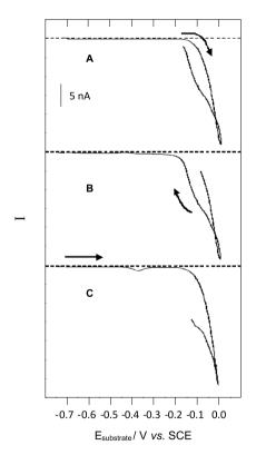
**Figure 5.** Consecutive tip-amperometric response obtained at the same time as cyclic voltammograms similar to voltammogram in Figure 4A. Tip held at  $-0.4\,V$ . (A) Forward scan with clean carbon fibre tip; (B) reverse scan and (C) forward scan with copper plated over the tip.
