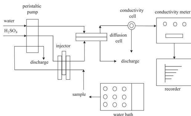
**Figure 1.** Diagram of the FIA/conductometric system used to determine the CO<sub>2</sub> concentration in toxicity assays.
