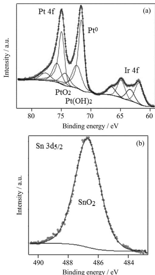
**Figure 3.** Fitted XPS core level spectra (a) Pt 4f and (b) Sn 3d<sub>5/2</sub> of the PtSnIr/C catalyst.
