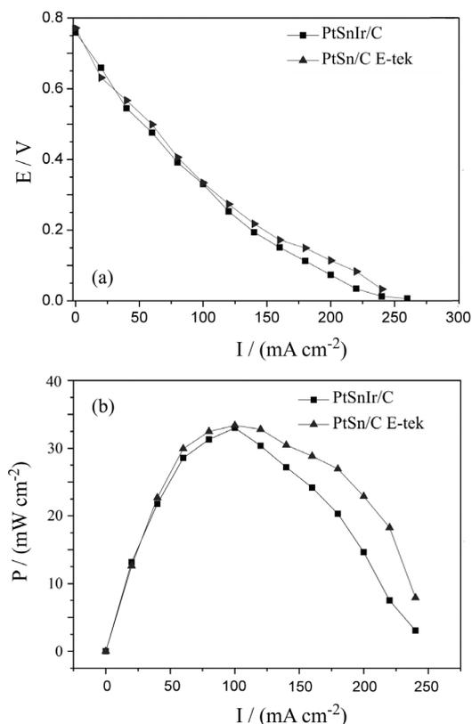
**Figure 4.** Polarization and power density curves in a 5 cm<sup>2</sup> DEFC at 100 °C using (a) PtSnIr/C (1 mg<sub>Pt+Ir</sub> cm<sup>-2</sup>) or 20 wt.% PtSnIr/C and (b) PtSn/C E-tek as anode catalysts (1 mg<sub>Pt</sub> cm<sup>-2</sup>) and 20 wt.% Pt/C E-tek as cathode catalyst (1 mg<sub>Pt</sub> cm<sup>-2</sup>). Nafion<sup>®</sup> 117 was used as membrane.
