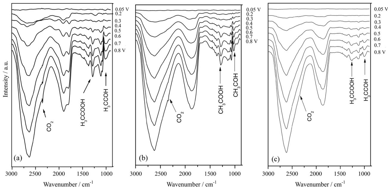
**Figure 5.** *In situ* FTIR spectra for a PtSnIr/C electrocatalyst in 0.1 mol L<sup>-1</sup> HClO<sub>4</sub> in the presence of ethanol at concentrations of (a) 0.5, (b) 1 and (c) 2 mol L<sup>-1</sup>. Reference spectra were taken at 0.05 V. Sample spectra measured after applying successive potential steps of 0.1 V, as indicated in the figure. Spectra were averaged from 128 scans. The spectral resolution was 8 cm<sup>-1</sup> using a SeZn prismatic window.
