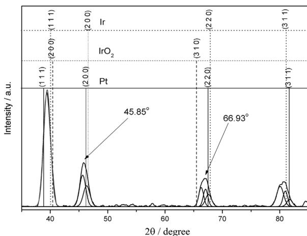
**Figure 2.** X-ray diffraction patterns of PtSnIr/C with the indicated peak patterns of Pt, Ir and IrO<sub>2</sub>.
