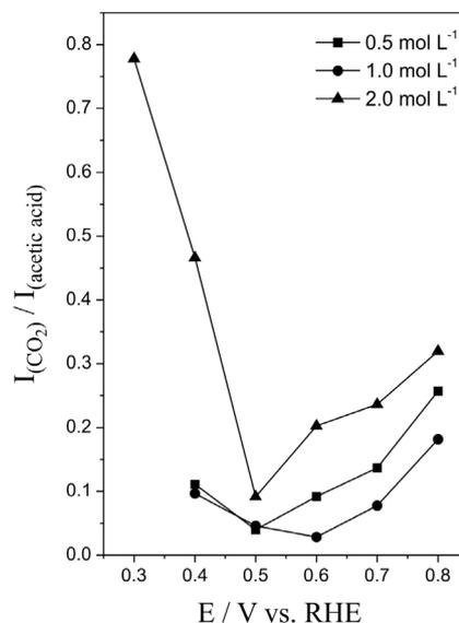
**Figure 7.** The ratio of integrated intensities of CO<sub>2</sub> and acetic acid as a function of potential for the three ethanol concentrations in the solutions.
