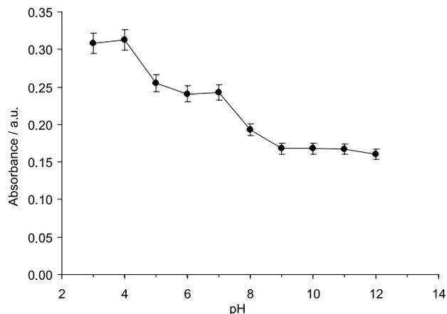
**Figure 1.** Effect of pH on the preconcentration and determination of cadmium. Conditions: 100  $\mu\text{g L}^{-1}$   $\text{Cd}^{2+}$ , 0.44% (m/v) of APDC, 60  $\mu\text{L}$   $[\text{Hmim}][\text{PF}_6]$  and extraction time 5 min.
