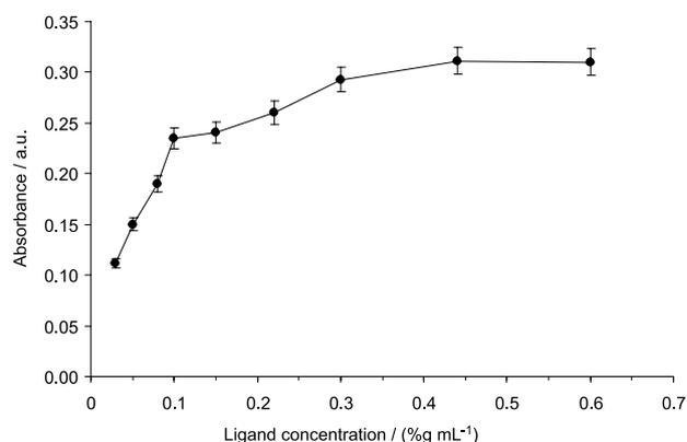
**Figure 2.** Effect of APDC concentration on the preconcentration and determination of cadmium. Conditions: pH: 3.8, 100  $\mu\text{g L}^{-1}$   $\text{Cd}^{2+}$ , 60  $\mu\text{L}$   $[\text{Hmim}][\text{PF}_6]$  and extraction time 5 min.
