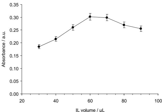
**Figure 3.** Effect of amounts of RTIL on the pre-concentration and determination of cadmium. Conditions: pH 3.8,  $100 \mu\text{g L}^{-1} \text{Cd}^{2+}$ ,  $0.44 \text{ (m/v)}$  of APDC and extraction time 5 min.
