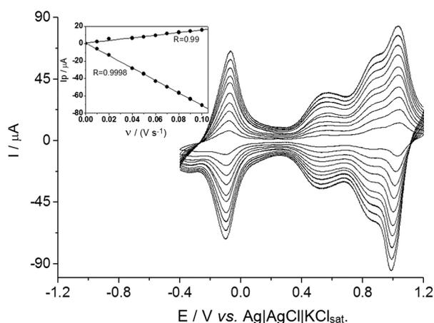
**Figure 2.** Cyclic voltammograms obtained at a glassy carbon electrode modified with a mixed film of ruthenium-based hexacyanoferrate at different scan rates (0.01 to 0.1 V s<sup>-1</sup>) in aqueous solution containing 0.1 mol L<sup>-1</sup> of Britton-Robinson buffer solution at pH 1.5. Inset figure: plot of anodic and cathodic peak currents vs. scan rate.
