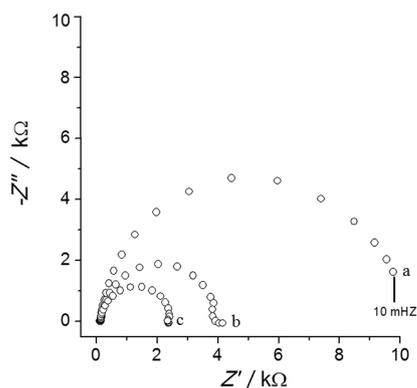
**Figure 7.** Nyquist plots for ethanol oxidation on glassy carbon electrode modified with a mixed film of ruthenium-based hexacyanoferrate in Britton-Robinson buffer solution at pH 1.5 with different concentrations of ethanol: (a) 0.1, (b) 0.5 and (c) 1.0 mol L<sup>-1</sup> at applied potential 0.98 V vs. Ag|AgCl|KCl<sub>sat</sub>.
