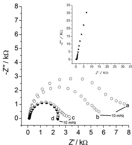
**Figure 6.** Complex-plane plots for ethanol oxidation on glassy carbon electrode modified with a mixed film of ruthenium-based hexacyanoferrate in Britton-Robinson buffer solution at pH 1.5 in the presence of 1.0 mol L<sup>-1</sup> ethanol at different applied potential: (a) 0.82, (b) 0.84, (c) 0.88 and (d) 0.98 V vs. Ag|AgCl|KCl<sub>sat</sub>. Inset figure: signal for modified electrode in supporting electrolyte in the absence of ethanol.
