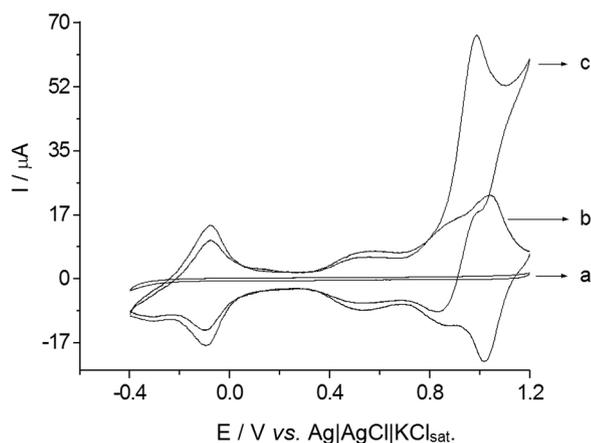
**Figure 4.** Cyclic voltammograms obtained at the bare glassy carbon electrode in the presence of ethanol (a), and at glassy carbon electrode modified with a mixed film of ruthenium-based hexacyanoferrate in Britton-Robinson buffer solution at pH 1.5 (b) in the absence and (c) presence of 0.1 mol L<sup>-1</sup> ethanol,  $v = 0.02$  V s<sup>-1</sup>.
