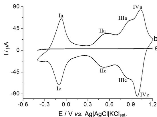
**Figure 1.** Cyclic voltammograms obtained at (a) bare glassy carbon electrode and (b) glassy carbon electrode modified with a mixed film of ruthenium-based hexacyanoferrate in  $0.1 \text{ mol L}^{-1}$  of Britton-Robinson buffer solution at pH 1.5,  $v = 0.1 \text{ V s}^{-1}$ .
