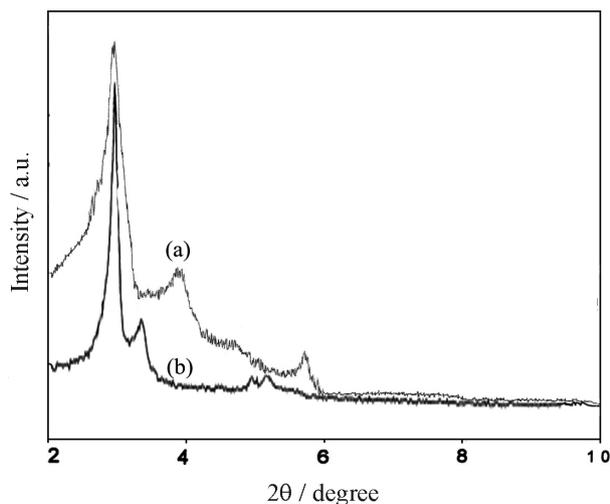
**Figure 3.** Low angle XRD patterns of (a) CoPc/MCM-48<sub>(hydrothermal)</sub> and (b) CoPc/MCM-41<sub>(hydrothermal)</sub>.
