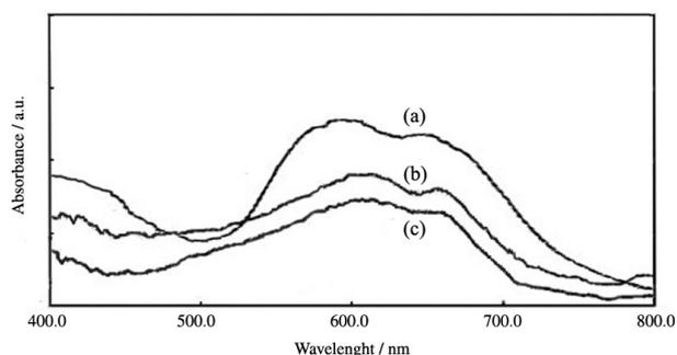
**Figure 5.** Diffuse reflectance spectra of (a) CoPc, (b) CoPc/MCM-48<sub>(hydrothermal)</sub> and (c) CoPc/MCM-41<sub>(hydrothermal)</sub>.
