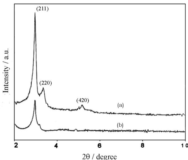
**Figure 2.** Low angle XRD patterns of (a) MCM-48<sub>(hydrothermal)</sub> and (b) CoPcS/NH<sub>2</sub>-MCM-48<sub>(hydrothermal)</sub>.
