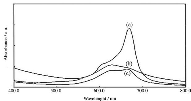
**Figure 4.** Diffuse reflectance spectra of (a) CoPcS, (b) CoPcS/NH<sub>2</sub>-MCM-48<sub>(hydrothermal)</sub> and (c) CoPcS/NH<sub>2</sub>-MCM-41<sub>(hydrothermal)</sub>.
