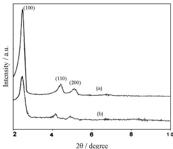
**Figure 1.** Low angle XRD patterns of (a) MCM-41<sub>(hydrothermal)</sub> and (b) CoPcS/NH<sub>2</sub>-MCM-41<sub>(hydrothermal)</sub>.
