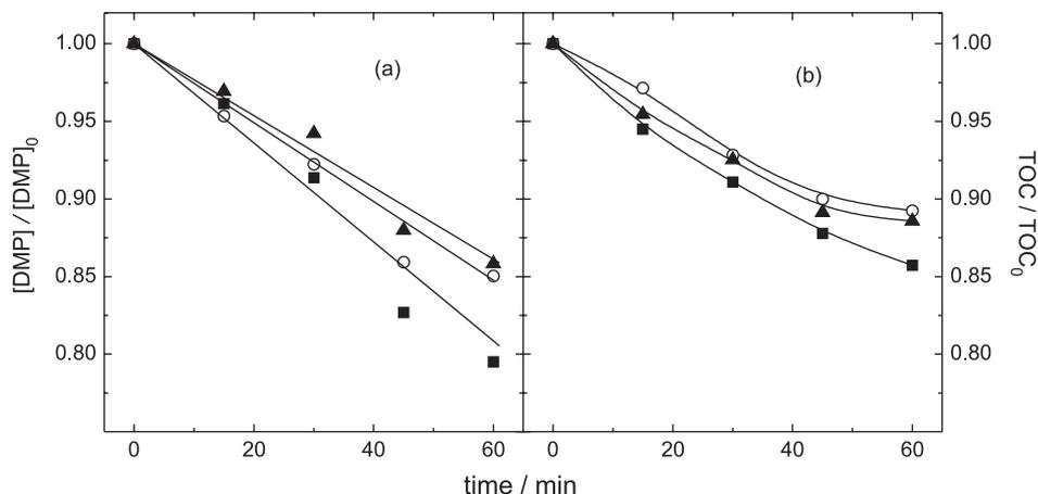
**Figure 3.** Relative DMP concentration and TOC decay as a function of the electrolysis time for different concentrations of NaCl: (■) 7, (○) 35, and (▲) 70 mmol dm<sup>-3</sup> NaCl. Conditions: 20 mA cm<sup>-2</sup>, 30 °C, and pH 2. Ionic strength of 0.15 mol dm<sup>-3</sup> through addition of Na<sub>2</sub>SO<sub>4</sub>.
