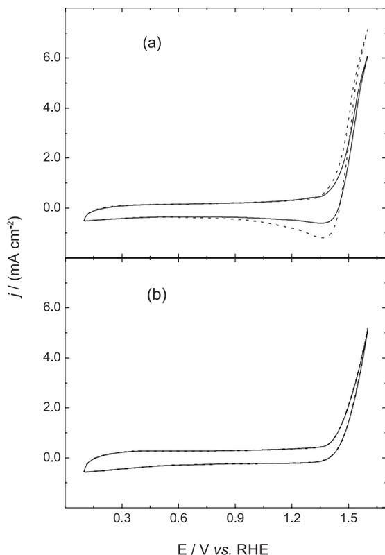
**Figure 2.** Cyclic voltammograms (10<sup>th</sup> cycle) of the commercial Ti/Ru<sub>0.3</sub>Ti<sub>0.7</sub>O<sub>2</sub> electrode at (a) 0.15 mol dm<sup>-3</sup> NaCl and (b) 0.05 mol dm<sup>-3</sup> Na<sub>2</sub>SO<sub>4</sub>, in the presence (dashed line) and absence (solid line) of DMP.  $v = 20 \text{ mV s}^{-1}$ . Ionic strength of 0.15 mol dm<sup>-3</sup>.
