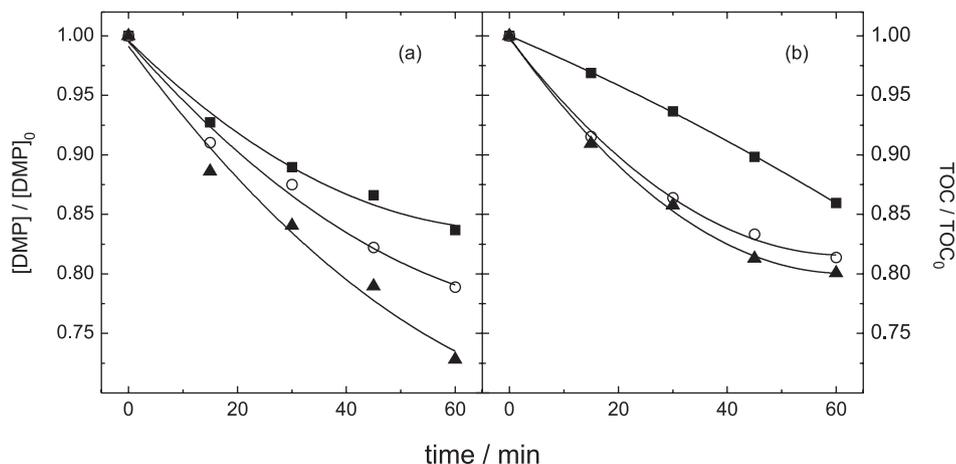
**Figure 6.** Relative DMP concentration and TOC decay as a function of the electrolysis time for different temperature values: (■) 10, (○) 30, and (▲) 50 °C. Conditions: 20 mA cm<sup>-2</sup>, pH 2, and 7.04 mmol dm<sup>-3</sup> NaCl. Ionic strength of 0.15 mol dm<sup>-3</sup> through addition of Na<sub>2</sub>SO<sub>4</sub>.
