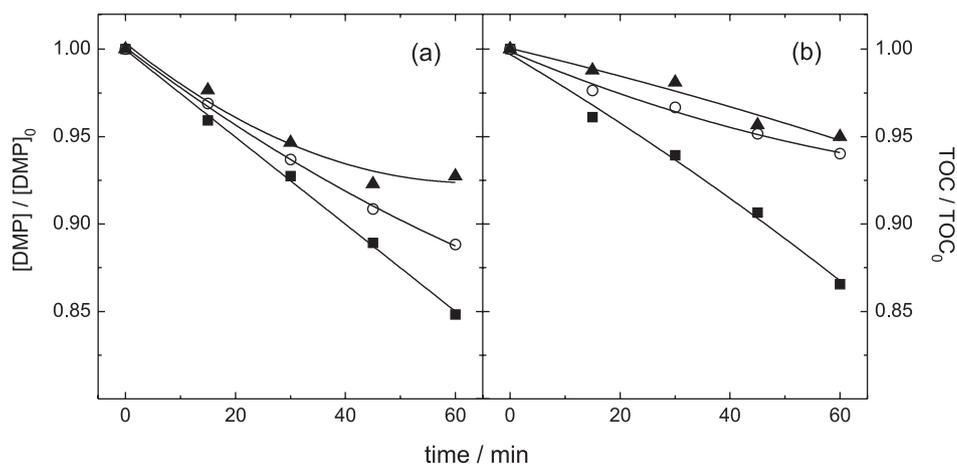
**Figure 4.** Relative DMP concentration and TOC decay as a function of the electrolysis time for different initial pH values: (■) pH 2, (○) pH 6, and (▲) pH 10. Conditions: 20 mA cm<sup>-2</sup>, 30 °C, and 7.04 mmol dm<sup>-3</sup> NaCl. Ionic strength of 0.15 mol dm<sup>-3</sup> through addition of Na<sub>2</sub>SO<sub>4</sub>.
