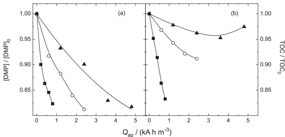
**Figure 5.** Relative DMP concentration and TOC decay as a function of the charge applied per unit volume of electrolyzed solution ( $Q_{ap}$ ) for different values of current densities: (■) 20, (○) 60, and (▲) 120 mA cm<sup>-2</sup>. Conditions: pH 2, 30 °C, and 7.04 mmol dm<sup>-3</sup> NaCl. The ionic strength was kept constant at 0.15 mol dm<sup>-3</sup> by addition of Na<sub>2</sub>SO<sub>4</sub>.
