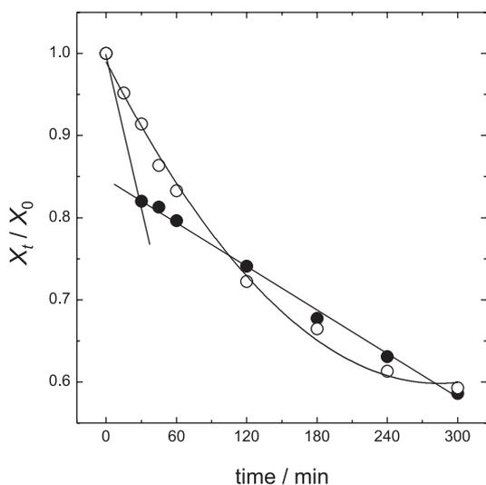
**Figure 7.** Relative (●) DMP concentration and (○) TOC decay as a function of the electrolysis time for the optimized conditions: 20 mA cm<sup>-2</sup>, 30 °C, pH 2, and 7.04 mmol dm<sup>-3</sup> NaCl. Constant ionic strength of 0.15 mol dm<sup>-3</sup> with the addition of Na<sub>2</sub>SO<sub>4</sub>.
