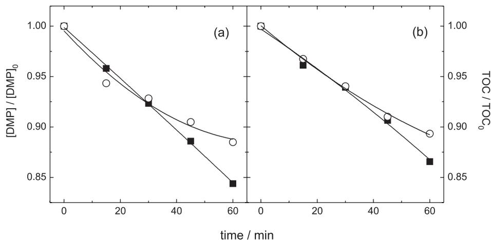
**Figure 1.** Relative DMP concentration and TOC decay as a function of the electrolysis time for different salt concentrations: 0.15 mol dm<sup>-3</sup> NaCl (■) and 0.05 mol dm<sup>-3</sup> Na<sub>2</sub>SO<sub>4</sub> (○). Conditions: 20 mA cm<sup>-2</sup>, 30 °C, and pH 2. Ionic strength of 0.15 mol dm<sup>-3</sup>.
