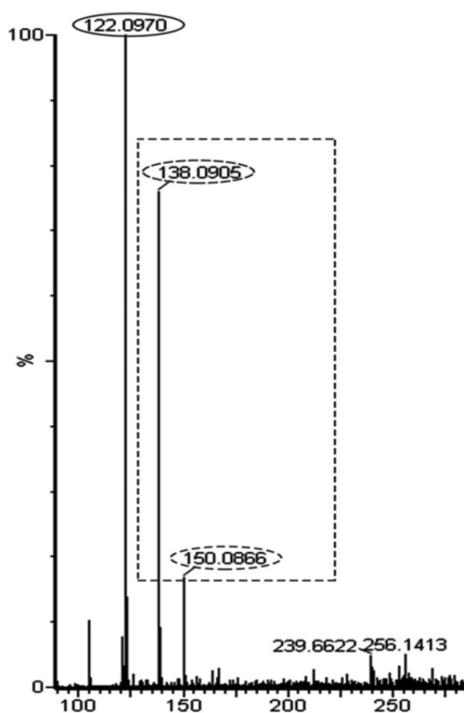
**Figure 3.** ESI-HRMS spectra for the aqueous solution of phenylethylamine irradiated at 5kGy for 170 min.
