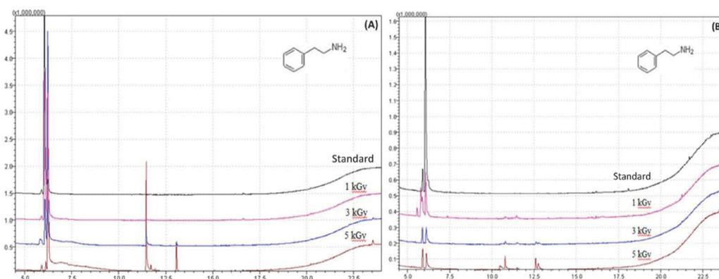
**Figure S1.** Chromatograms of the methanolic (A) and aqueous (B) solutions of phenylethylamine after irradiation at different doses. Mode: scan; Column: RTX-5MS (5% diphenyl/95% dimethyl polysiloxane); Ramp: 2 min, 80 °C; 10 °C min<sup>-1</sup>, 80 °C to 280 °C.
