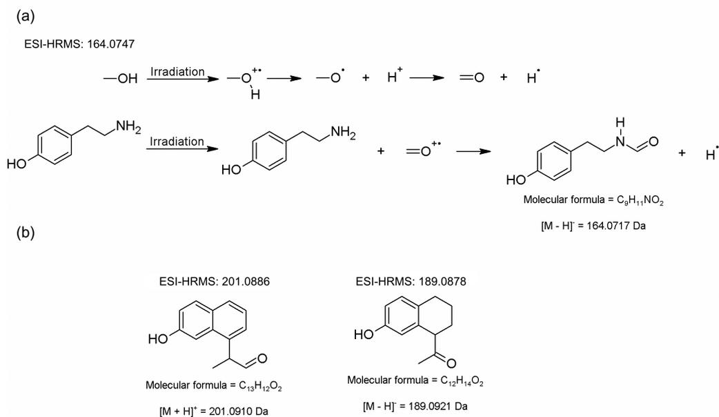
**Figure 5.** (a) Proposed structures of the main radiolytic products of the methanolic solution of tyramine and possible mechanistic schemes for their formation and (b) proposed structures of the radiolytes of tyramine irradiated in aqueous solution according to the exact mass encountered.
