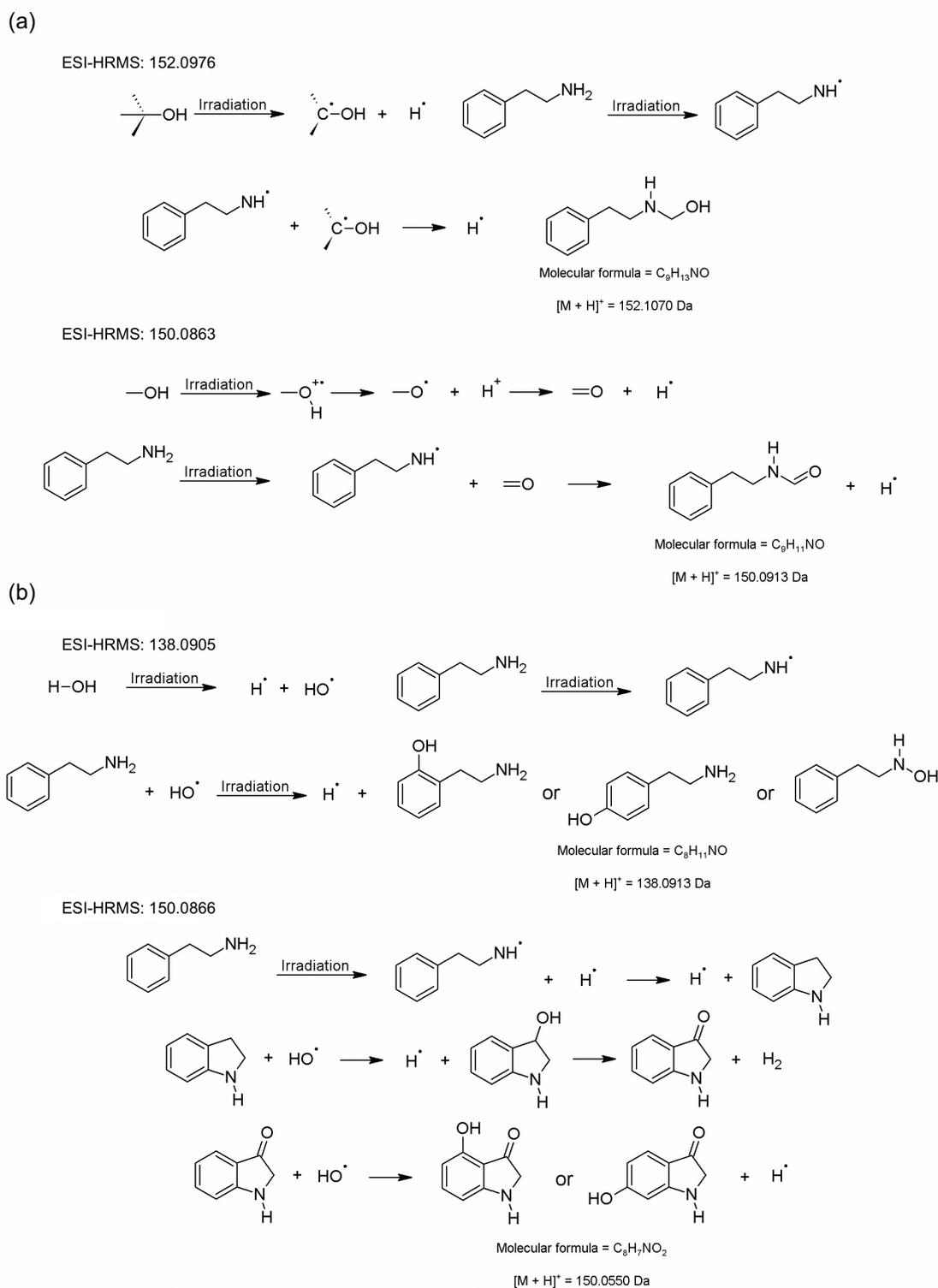
**Figure 2.** Proposed structures of the main radiolytic products of the methanolic (a) and aqueous (b) solutions of phenylethylamine and possible mechanistic schemes for their formation.
