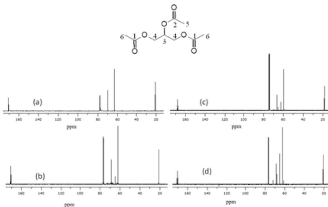
**Figure 2.**  $^{13}\text{C}$  NMR (a) standard triacetin; (b) triacetin 1:6 (glycerol:acetic acid and A-15); (c) triacetin 1:3 (glycerol:acetic anhydride with A-15); (d) triacetin 1:6 (glycerol:acetic acid and  $\text{H}_2\text{SO}_4$ ).
