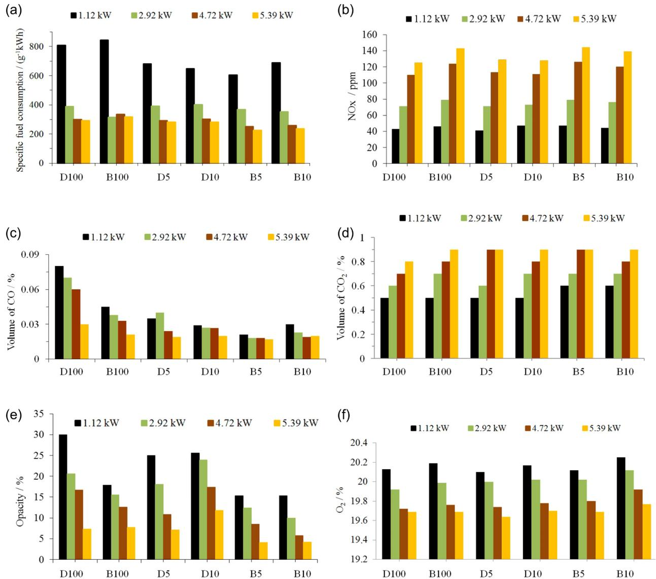
**Figure 3.** (a) Specific fuel consumption vs. engine speed; (b) NO<sub>x</sub> emission; (c) CO emission; (d) CO<sub>2</sub> emission; (e) opacity emission and (f) O<sub>2</sub> emission.
