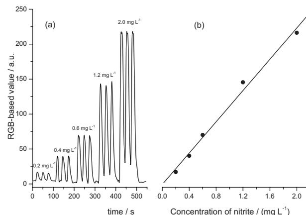
**Figure 5.** (a) Transient signals; (b) calibration curve for determination of the 0.2-2.0 mg L<sup>-1</sup> NO<sub>2</sub><sup>-</sup>, using detection by webcam.
