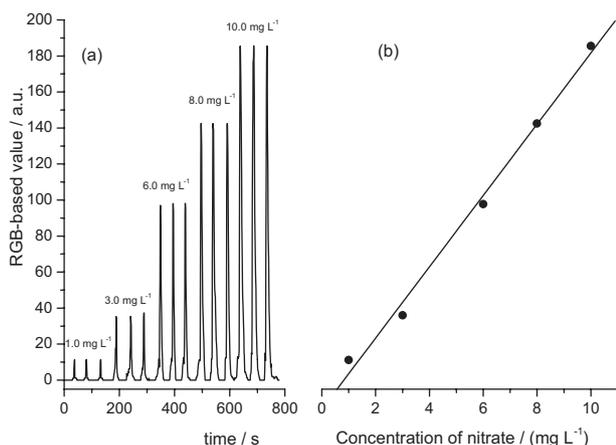
**Figure 6.** (a) Transient signals; (b) calibration curve for determination of the 1.0-10.0 mg L<sup>-1</sup> NO<sub>3</sub><sup>-</sup>, using detection by webcam.
