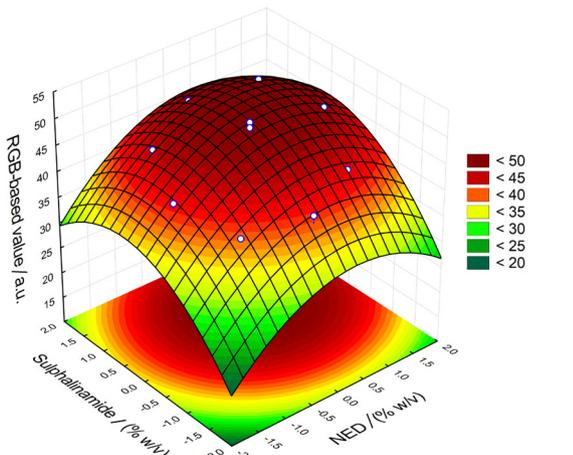
**Figure 4.** Central composite design of sulphalamide and NED concentration.  $RGB\text{-based value} = 49.67 + 2.19NED - 2.46(NED)^2 + 2.86(\text{sulphalamide}) - 2.71(\text{sulphalamide})^2 + 0.25(NED)(\text{sulphalamide})$ .
