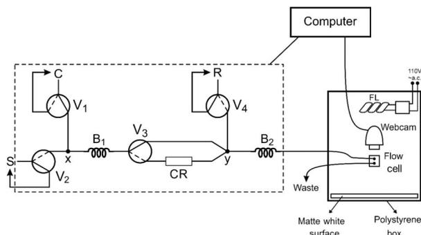
**Figure 1.** Flow diagram of the system for nitrite and nitrate determination. V<sub>1</sub>-V<sub>4</sub>: solenoid valves; C: buffer solution (pH = 7.2) (4.3 mL min<sup>-1</sup>); S: sample (4.3 mL min<sup>-1</sup>); R: Griess reagent (2.1 mL min<sup>-1</sup>); CR: Cd reduction mini-column (3 mm i.d. × 6 cm); B<sub>1</sub> (0.8 mm i.d. × 60 cm) and B<sub>2</sub> (0.8 mm i.d. × 90 cm): coiled reactors; x and y: confluence sites; FL: fluorescent lamp; webcam: detector.
