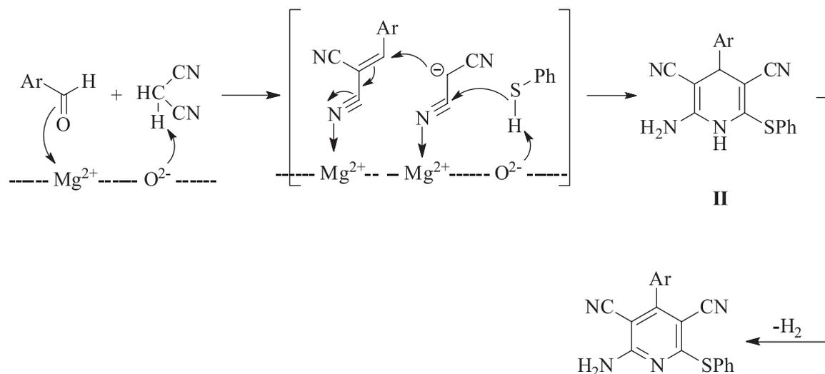
**Scheme 2.** Synthesis of compound **4** in the presence of MgO as catalyst.
