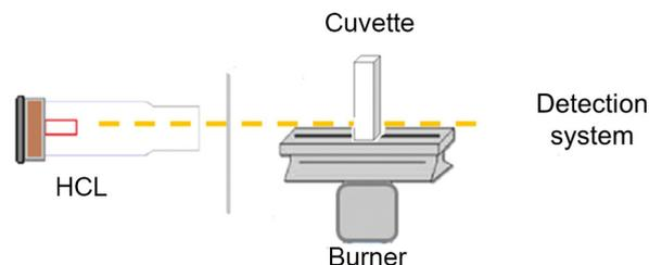
**Figure 1.** Illustration of the system used for determination of caffeine at 271.9 nm and propranolol at 285.2 nm on an atomic absorption spectrometer using Fe and Mg hollow cathode lamps, respectively.
