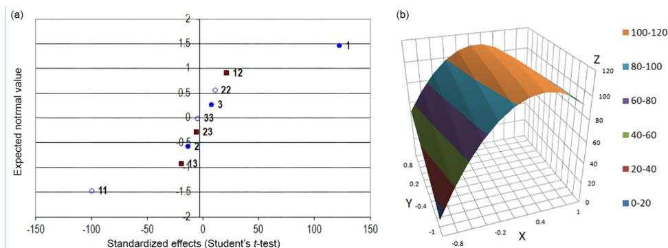
**Figure 1.** Influence of HNO<sub>3</sub> and time on the extraction of elemental sulfur assisted by microwave radiation; (a): normal probability; (b) surface response. In (b) the x-axis corresponds to the volume of HNO<sub>3</sub> added (in steps), y-axis to the time of extraction (in steps) and z-axis to the S concentration in % (m/m).
