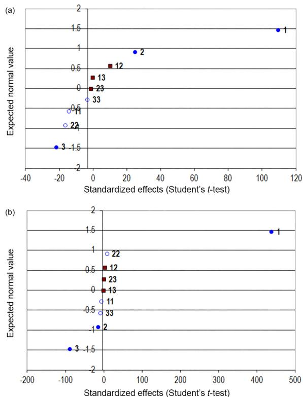
**Figure 2.** Average probability for (a) S and (b)  $Mg^{II}/Mg^I$  ratio. The first factor is the plasma power, the second the peristaltic pump speed and the third the nebulizer gas pressure. The other effects shown are contributions of second order.
