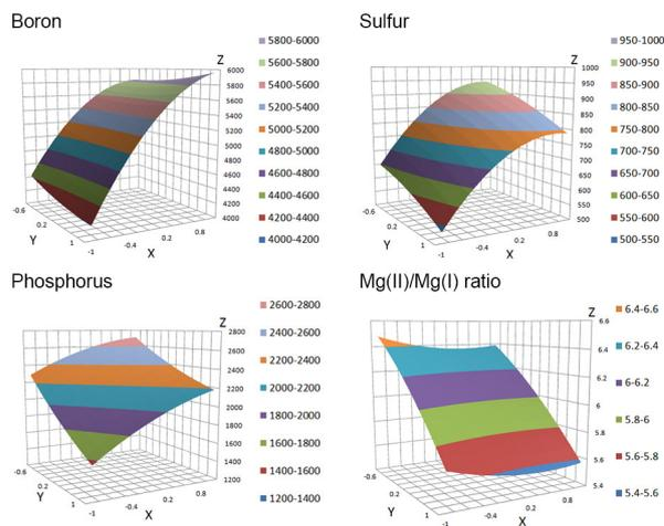
**Figure 3.** Response surface of the instrumental conditions; X corresponds to the peristaltic pump speed (in matrix coordinates), Y the nebulizer gas pressure (in matrix coordinates) and Z the intensity of the analyte signal, except  $Mg^{II}/Mg^I$  where Z corresponds to this ratio.
