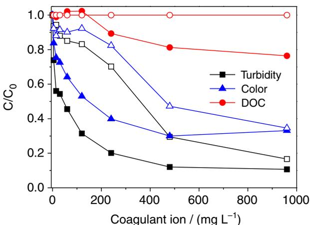
**Figure 2.** Effect of dosage of coagulant ion on the removal of turbidity, apparent color and DOC from raw landfill leachate by coagulation-flocculation using  $\text{Fe}^{3+}$  (solid symbols) and  $\text{Al}^{3+}$  (open symbols).
