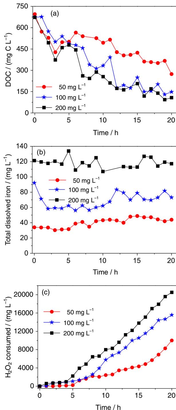
**Figure 1.** Effect of  $\text{Fe}^{2+}$  concentration on (a) DOC removal; (b) concentration of total dissolved iron; (c)  $\text{H}_2\text{O}_2$  consumption, during the raw landfill leachate treatment by the photo-Fenton process. Initial conditions:  $\text{DOC} = 680 \pm 13 \text{ mg C L}^{-1}$ ;  $\text{H}_2\text{O}_2 = 2000 \text{ mg L}^{-1}$  (replaced when close to  $200 \text{ mg L}^{-1}$ );  $\text{pH} = 2.5\text{-}2.8$ .
