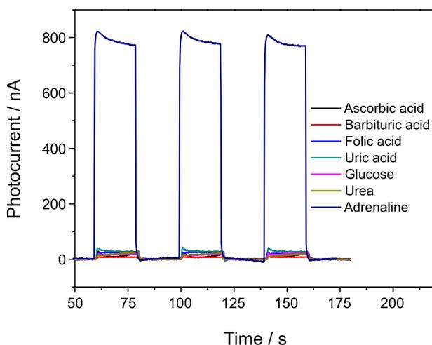
**Figure 7.** Photocurrent obtained for proposed photoelectrochemical sensor toward several foreign species in comparison to that obtained for adrenaline under optimized conditions at an applied potential of 0.4 V vs. Ag/AgCl. The concentration of all species was fixed at 100  $\mu\text{mol L}^{-1}$ .
