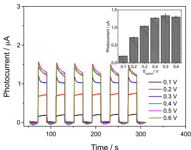
**Figure 5.** Influence of applied potential on the photocurrent for  $100 \mu\text{mol L}^{-1}$  of adrenaline. Measurements were carried out in  $0.1 \text{ mol L}^{-1}$  phosphate buffer solution.
