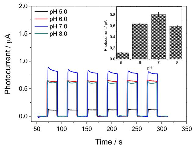
**Figure 4.** Influence of pH of the solution on the photosensor response for  $100 \mu\text{mol L}^{-1}$  adrenaline. Measurements were carried out in  $0.1 \text{ mol L}^{-1}$  phosphate buffer solution.  $E_{\text{app}} = 0.25 \text{ V vs. Ag/AgCl}$ .
