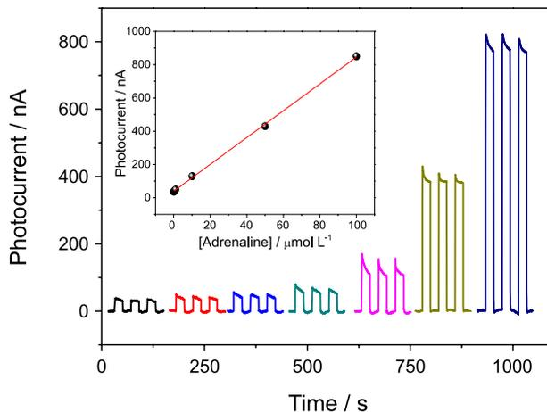
**Figure 6.** Photocurrent of photoelectrochemical sensor obtained under optimized conditions to adrenaline concentrations between  $0.01$  and  $100 \mu\text{mol L}^{-1}$ . Inset: analytical curve.
