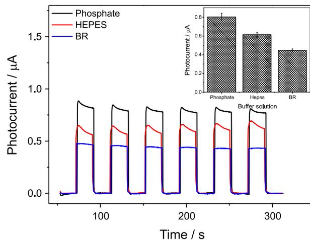
**Figure 3.** Influence of buffer solution on the photosensor response for  $100 \mu\text{mol L}^{-1}$  of adrenaline. Measurements were carried out in  $0.1 \text{ mol L}^{-1}$  phosphate buffer solution.  $E_{\text{app}} = 0.25 \text{ V vs. Ag/AgCl}$ .
