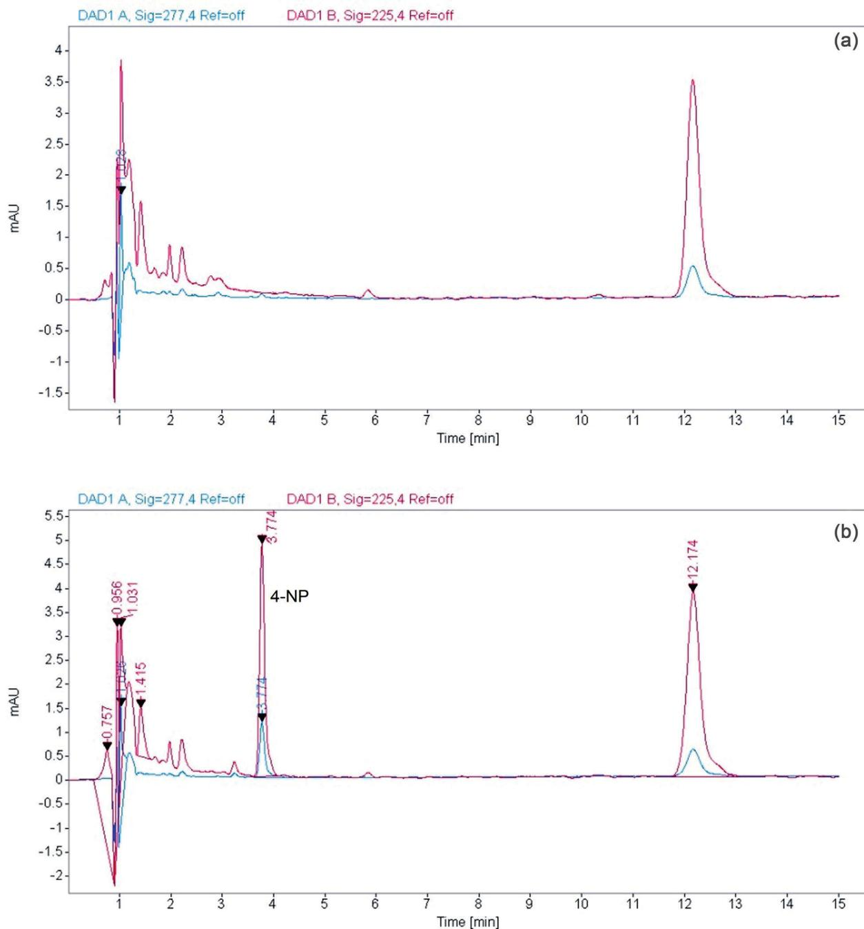
**Figure 2.** Chromatogram with optimized conditions of the (a) blank (matrix only) and (b) synthetic sample (matrix and 4-nonylphenol).
