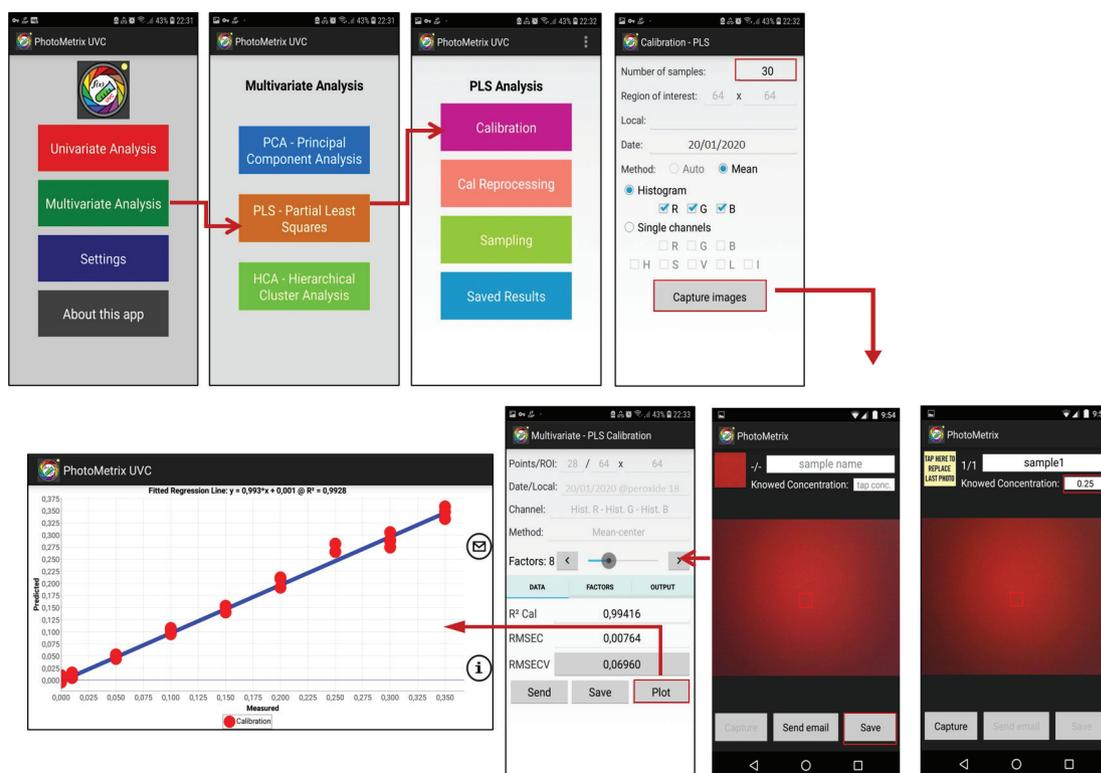
Figure 2. Main graphic interface of the PhotoMetrix UVC application for the PLS calibration model.
