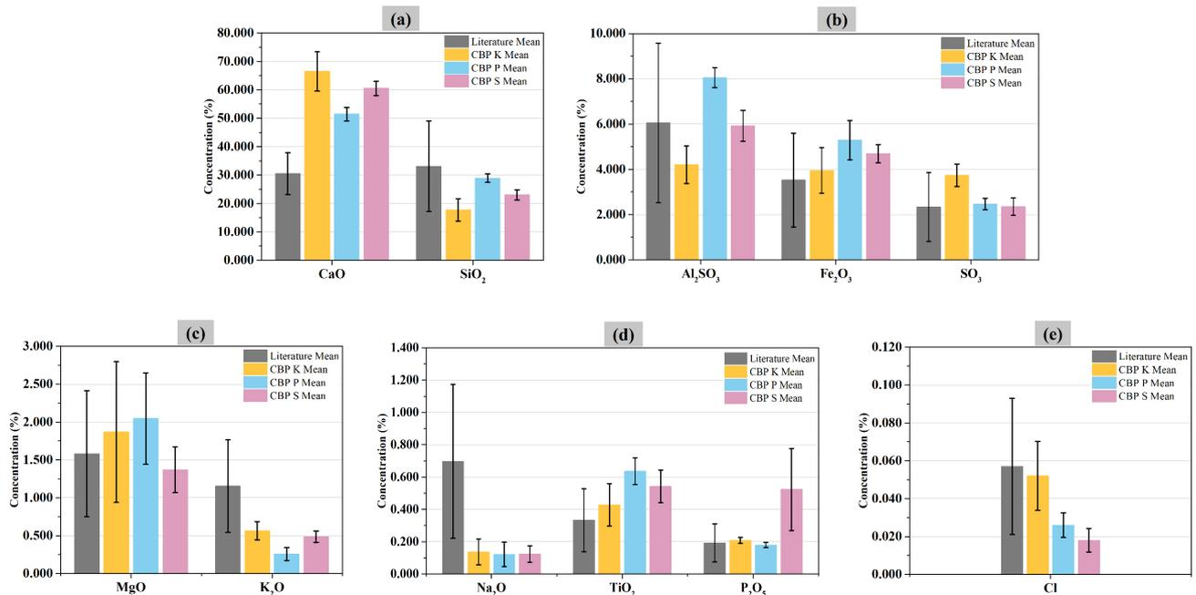
Figure 8. Average of the contents of oxides and elements common between CBP and literature.
