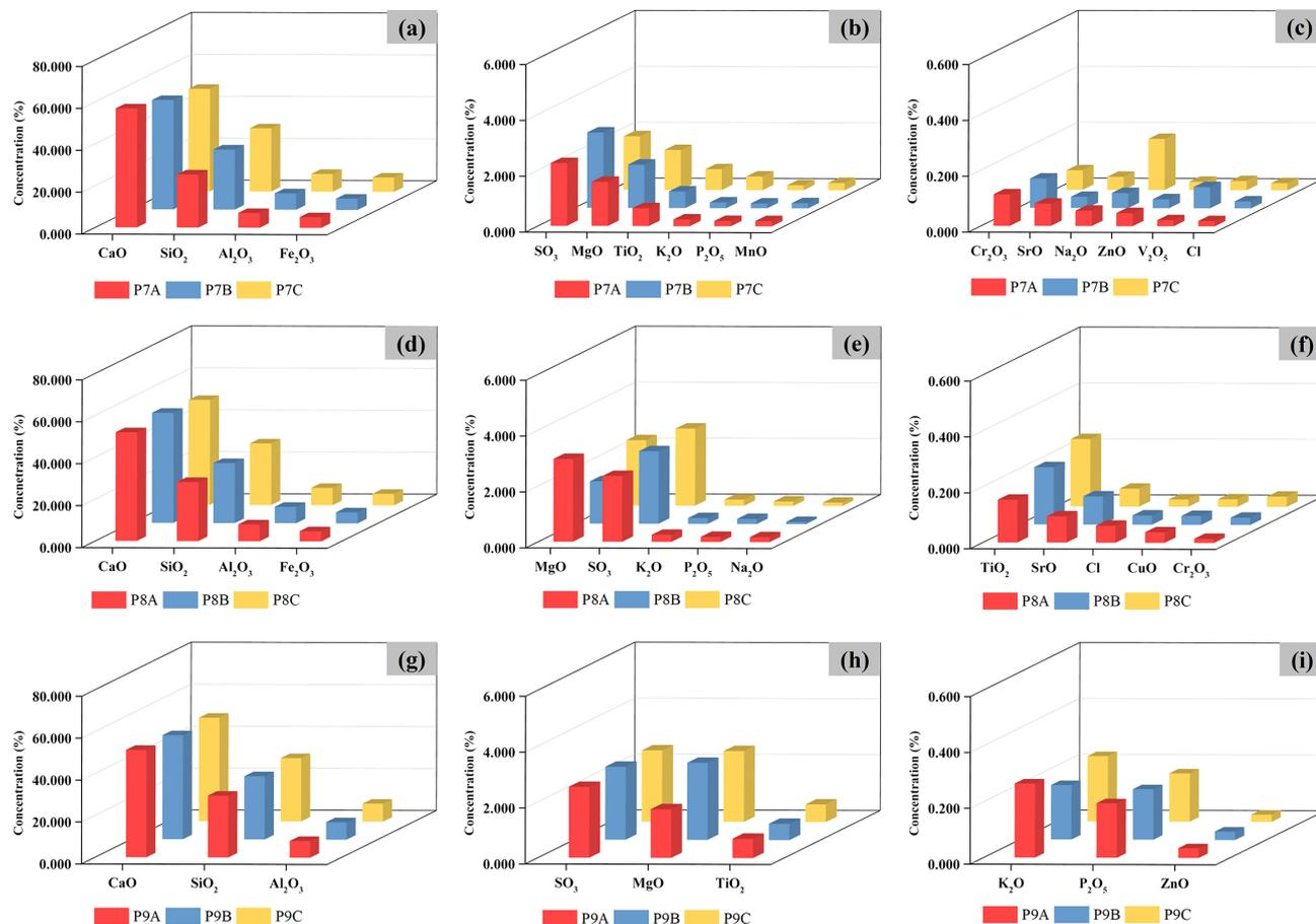
**Figure 3.** Average concentration of elements and oxides *per* collection point at CBP P: (a), (b) and (c) in month 7; (d), (e) and (f) at month 8; (g), (h) and (i) in month 9.
