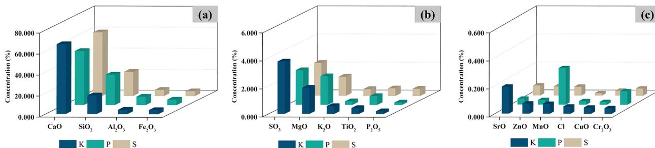
**Figure 6.** Average concentration of elements and oxides of the three CBP: (a) CaO, SiO<sub>2</sub>, Al<sub>2</sub>O<sub>3</sub> and Fe<sub>2</sub>O<sub>3</sub> in the CBP K, P and S; (b) SO<sub>3</sub>, MgO, K<sub>2</sub>O, TiO<sub>2</sub> and P<sub>2</sub>O<sub>5</sub> in the CBP K, P and S; (c) SrO, ZnO, MnO, Cl, CuO, Cr<sub>2</sub>O<sub>3</sub> in the CBP K, P and S.
