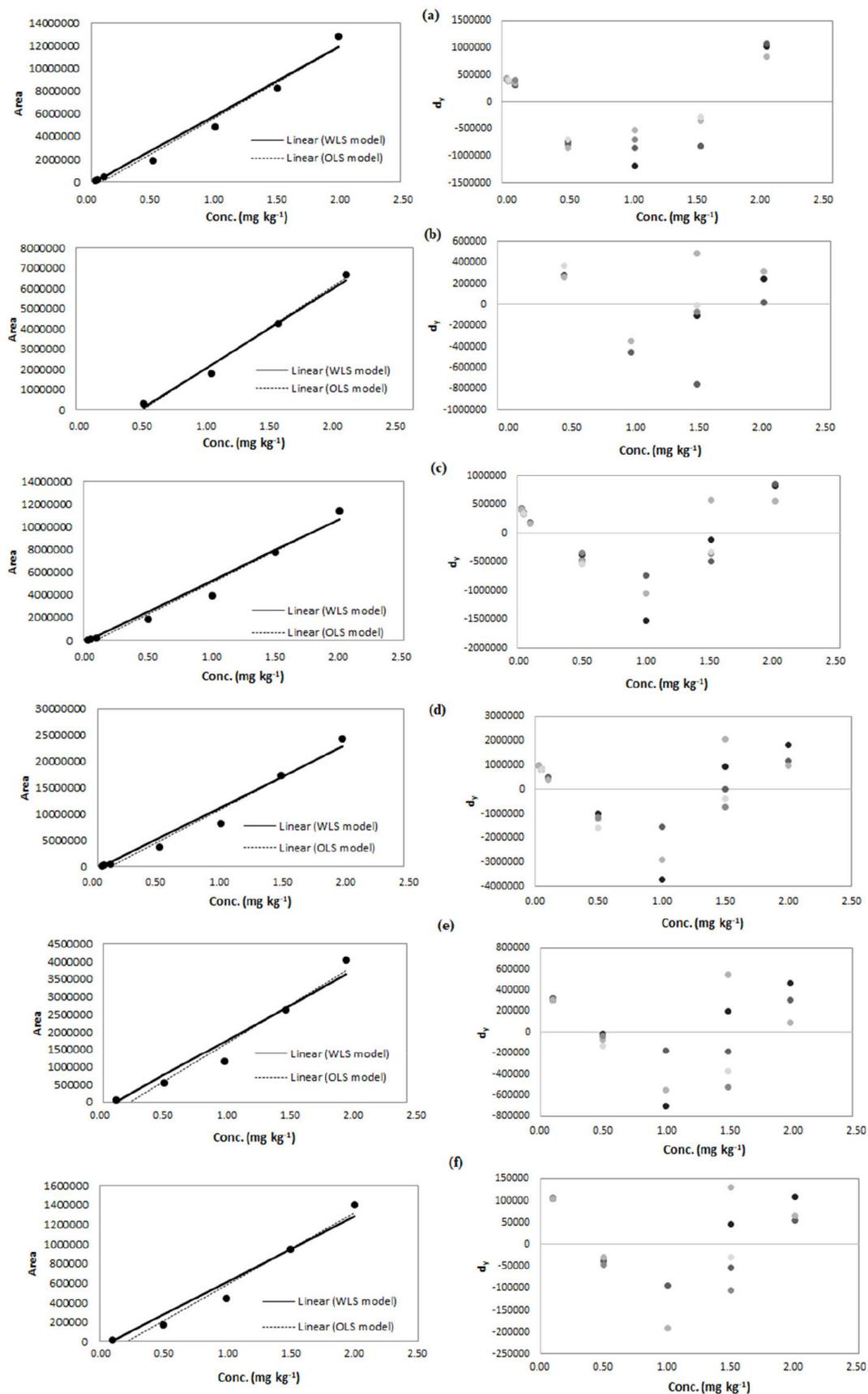
**Figure 2.** Analytical curves (OLS and WLS models) and residuals graphs obtained by statistical analysis of linearity: (a) trifluralin, (b) chlorothalonil, (c) chlorpyrifos, (d) bifenthrin, (e) pyriproxyfen, (f) cyfluthrin.
