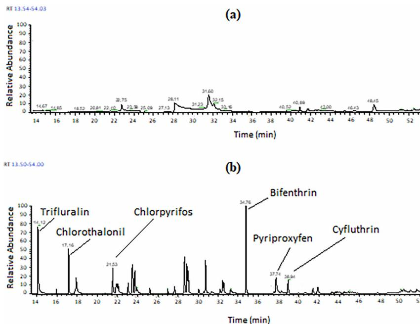
**Figure 1.** Chromatogram of (a) tomato matrix blank; (b) standard solution of pesticides (2 mg kg<sup>-1</sup>) in the matrix.
