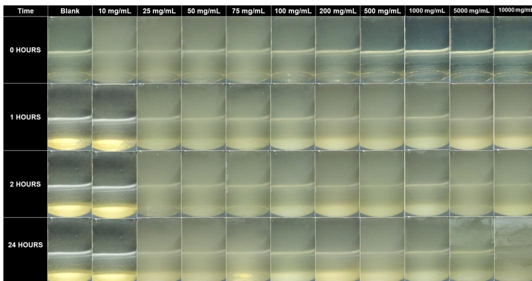
**Figure 2.** The visual appearance of the self-precipitating mixed brines and scale inhibitor brines in the chemical compatibility test at 65 °C, with Fe<sup>III</sup> ion.
