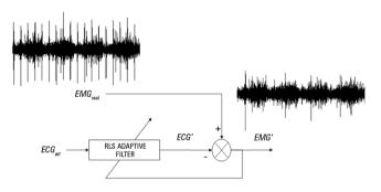
**Figure 1** - Scheme of the adaptive filter process using RLS algorithm. Where EMGreal is the recorded EMG signal that was bandpass filtered, ECGart is an artificial ECG signal obtained from EMGreal, ECG' is the ECG obtained from adaptive filter and EMG' is the EMG with a reduced cardiac interference.  $\text{EMG}_{\text{real}}$  - real electromyogram; ECG<sub>ur</sub> - artificial electrocardiogram; ECG - electrocardiogram.
