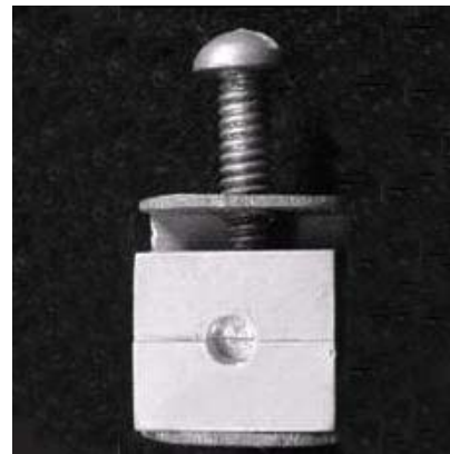
Figure 3. Matrix used for the Knoop hardness test.
