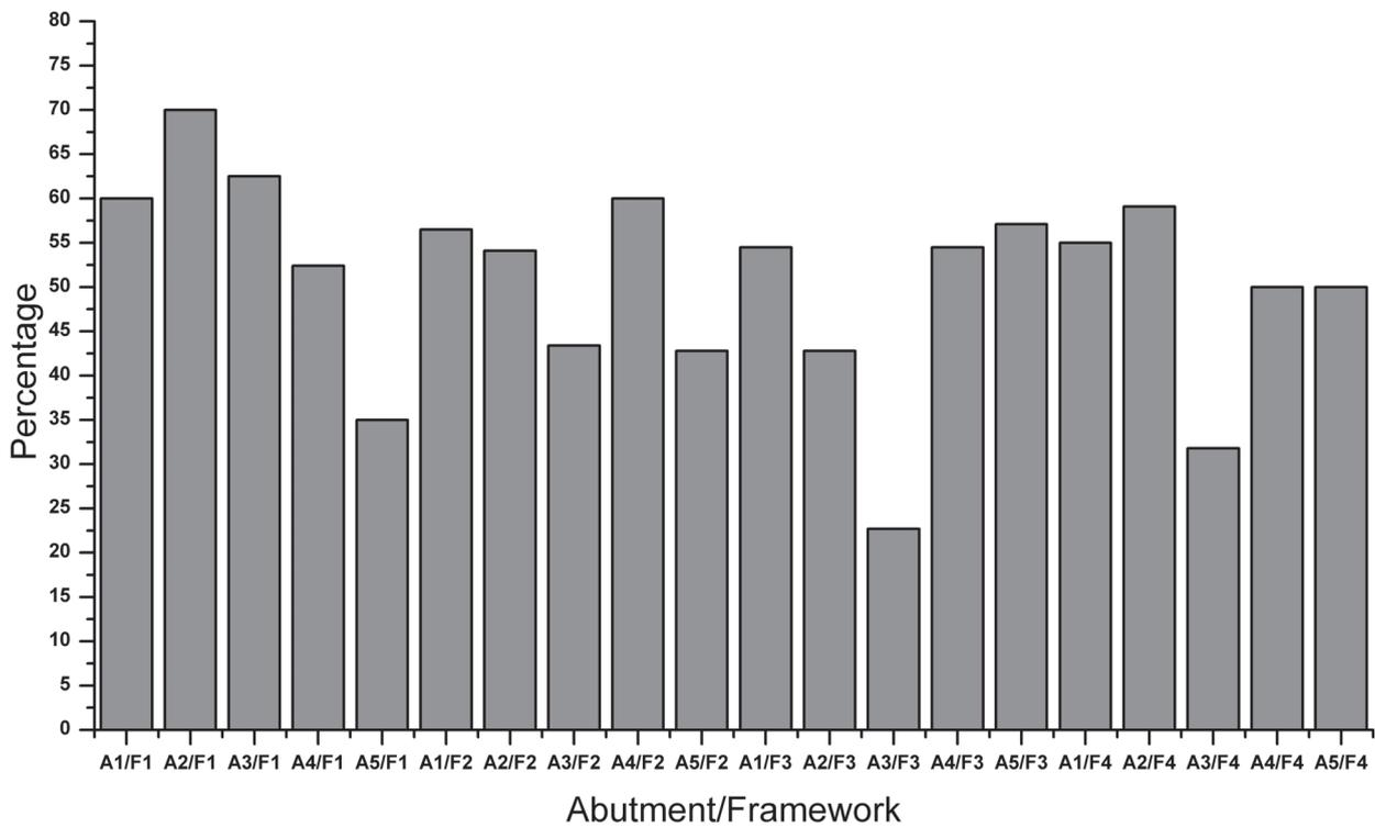
Figure 4. Percentage of torque loss values between each abutment and the CP Ti framework.
