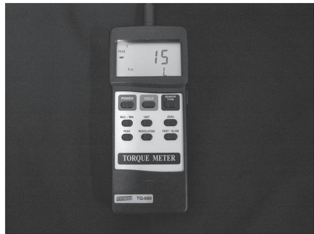
Figure 2. Detorque value registered in the digital torque meter.
