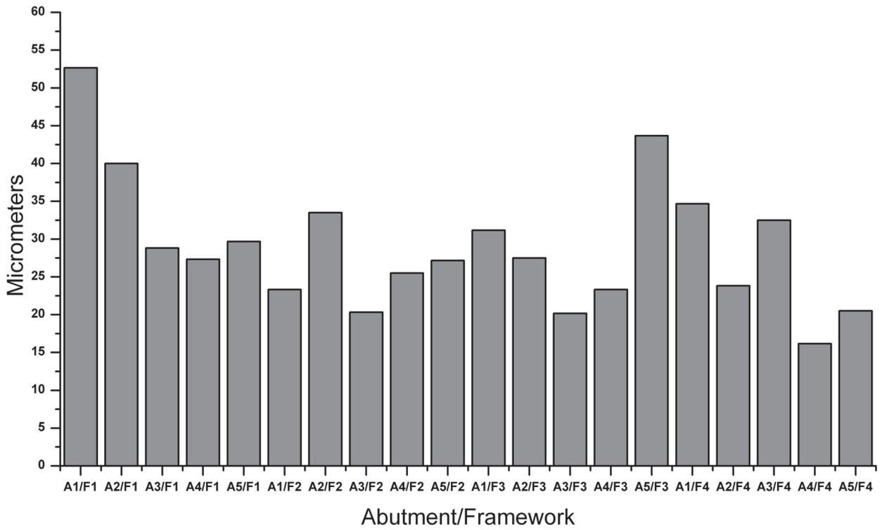
Figure 3. Vertical misfit between each abutment and the CP Ti framework.
