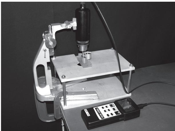
Figure 1. Torque application with the digital torque meter.
