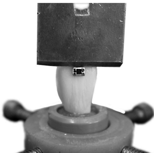
Figure 1. Bovine incisor with metallic bracket bonded to buccal enamel and the active chisel tip acting on the upper part of the bracket base during the shear bond strength test.
