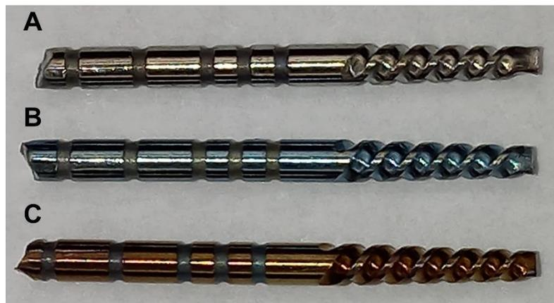
Figure 1. Images of (A) Conventional ProFile instruments, (B) Blueish ProFile instruments after  $500\text{ }^{\circ}\text{C}$  heat treatments, and (C) Yellowish ProFile instruments after  $450\text{ }^{\circ}\text{C}$  heat treatments.
