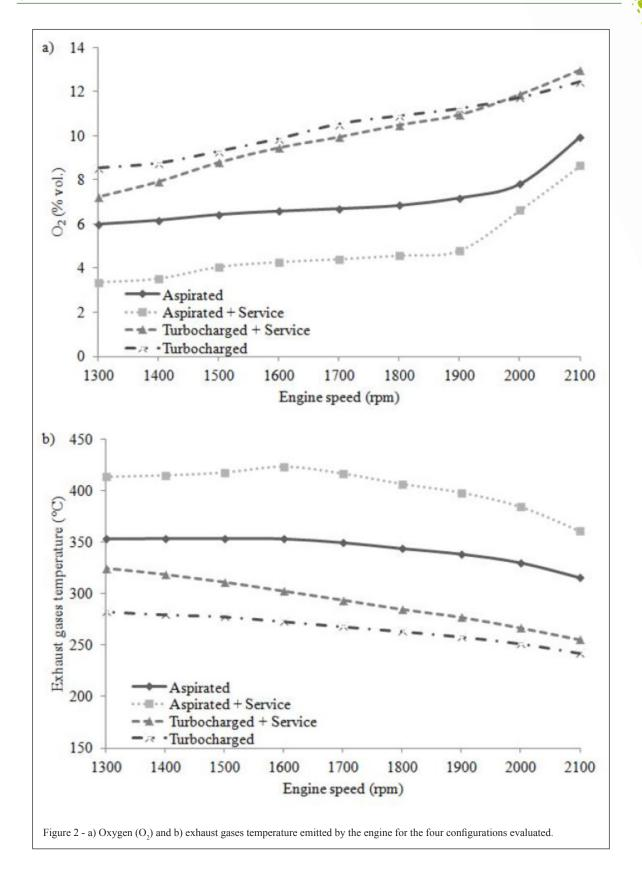
for configurations C1, C2, C3 and C4 were 353.00; 422.67; 324.33; and 282.67°C, respectively. One can observe that these temperatures happened close to the engine maximum torque rotations. Considering the exhaust gases temperature behavior, there is an increase in the temperature when the loads applied to the engine are higher (AGARWAL et al., 2007).
