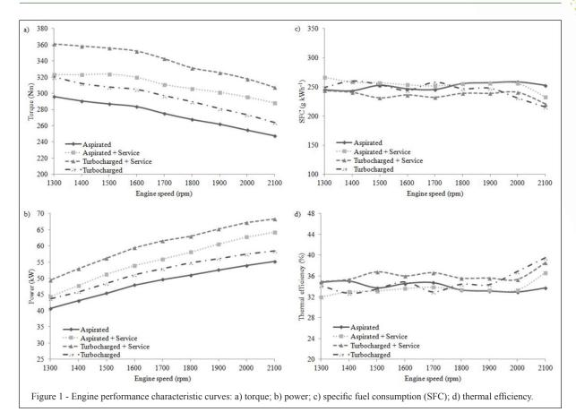
The best air/fuel ration mixed in the engine's combustion chamber can cause the reduction of the specific fuel consumption of the engine working at C3 configuration. The specific fuel consumption decreases due to the air temperature elevation and the increase of air mass inside the cylinder, ensuring the injected Diesel oil combustion. Thus, the best burn of this mixture favors the increase of engine power and; consequently, reduced the specific fuel consumption (KARABEKTAS, 2009).
