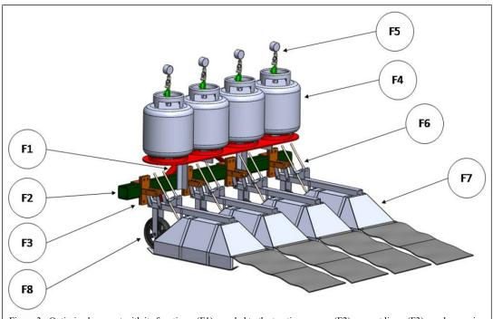
Figure 3 - Optimized concept with its functions: (F1) coupled to the traction source, (F2) support lines, (F3) regular spacing between the lines, (F4) storage gas, (F5) dosing gas, (F6) apply heat, (F7) heat insulation, (F8) regulate height.
