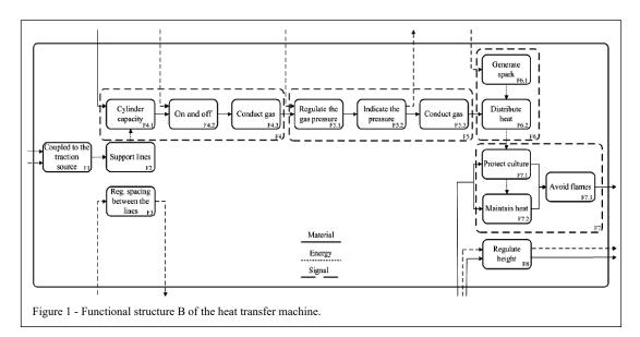
point coupling should be in accordance with NBR 730 in order to fit into categories 1 and 2. The function "support lines" (F2) refers to the support mechanism for the connection of the lines since the "regular spacing between the lines" function (F3) determines that the machine should present a variation between a line as well as the junction of two lines allowing the control of weeds in different crops according to project specifications defined by SPAGNOLO et al. (2018).
