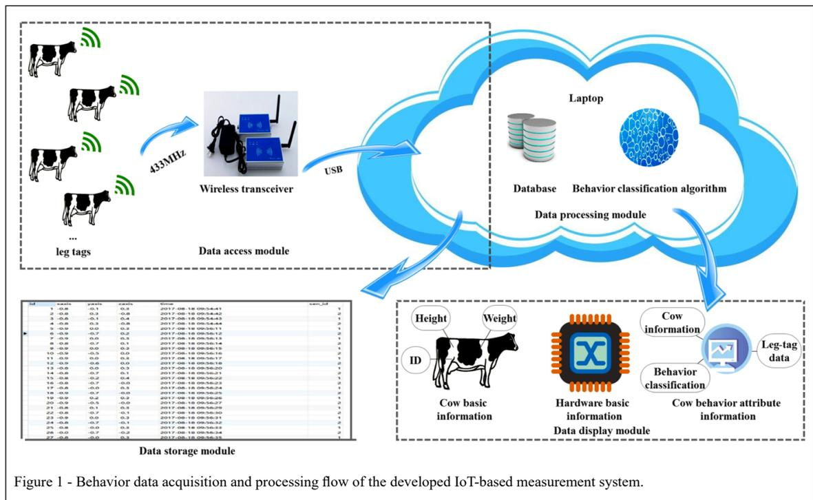
Figure 1 - Behavior data acquisition and processing flow of the developed IoT-based measurement system.
