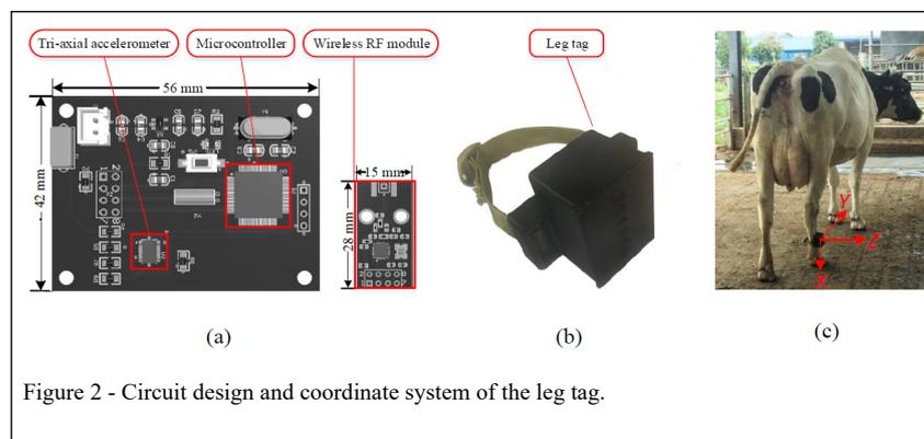
Figure 2 - Circuit design and coordinate system of the leg tag.
