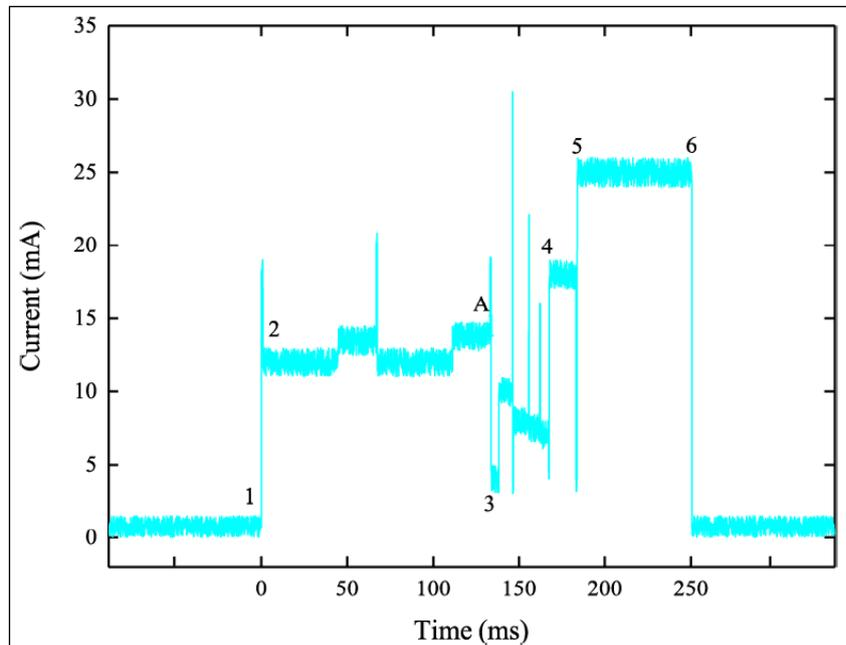
Figure 6 - Current consumption during one measurement and transmission cycle.
