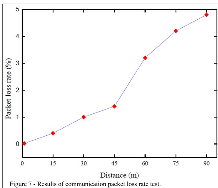
Figure 7 - Results of communication packet loss rate test.
