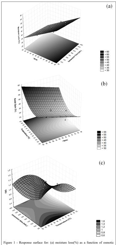
Figure 1 - Response surface for: (a) moisture loss(%) as a function of osmotic solution concentration (°Brix) and immersion time (minutes); (b) solid gain(%) as a function of osmotic solution concentration (°Brix) and temperature (°C); and (c) Dehydration efficiency index(DEI) as a function of temperature (°C) and immersion time(minutes).
