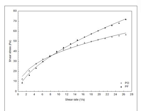
Figure 4 - Fitting ability of Power Law model to experimental steady shear flow curve of psyllium mucilage.
