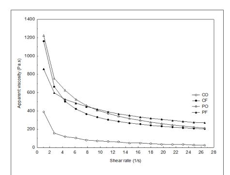
Figure 2 - Effect of different methods on apparent viscosity of chia and psyllium mucilage as a function of shear rate, at 25 °C for samples CO, CF, PO and PF. CO (chia mucilage dried in oven), CF (chia mucilage dried in freeze dryer), PO (psyllium mucilage dried in oven) and PF (psyllium mucilage dried in freeze dryer).
