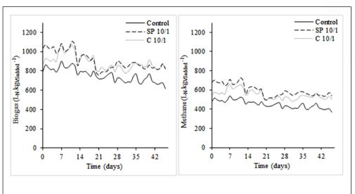
Figure 1 - Specific production of biogas and methane by VS<sub>added</sub> during the 47-day period.
