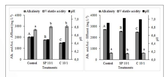
Figure 2 - Alkalinity (mg CaCO<sub>3</sub> L<sup>-1</sup>), volatile acidity (mg L<sup>-1</sup>), and pH in the affluent and effluent in semi-continuous digesters in the anaerobic co-digestion of swine manure (SM), sweet potato (SP), and cassava (C). Distinct letters above the bars differ by Tukey test (P<0.05).
