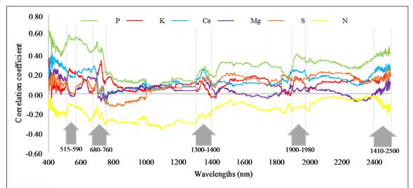
Figure 6 - Spearman's coefficient of correlation between Nitrogen (N), Phosphorus (P), Potassium (K), Calcium (Ca), Magnesium (Mg) and Sulfur (S) in the leaves and reflectance in the wavelengths between 400 and 2500 nm for the harvest 2020/21. Spectral regions with the greatest correlation variations in the ranges of Visible (515-590 nm), Red-Edge (680-760 nm) and Mid-Infrared (1300-1400 nm,1900-1980 nm and 1410-2500 nm) were also identified.
