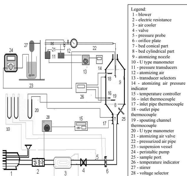
Figure 1 - Experimental apparatus.
