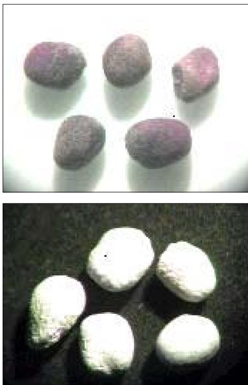
Figure 4 - Microscope view (40x) of non-coated broccoli seeds (a) and broccoli seeds coated in spouted bed (b).
