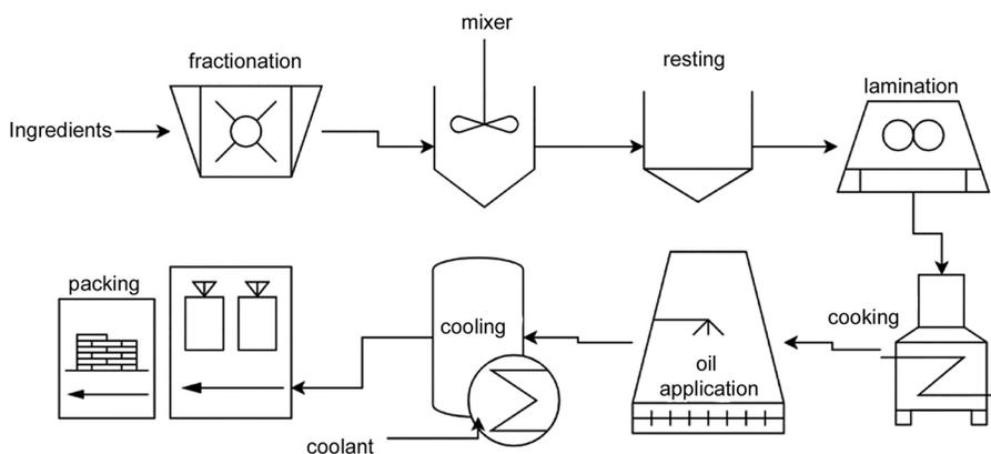
**Figure 1** – Flowchart of appetizer-type Mignon cracker's production on industrial scale.
