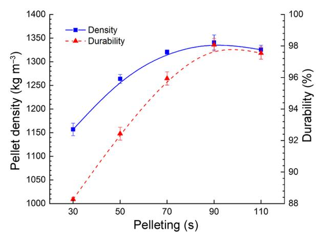
Figure 5 – Pellet density and durability with different pelleting times.
