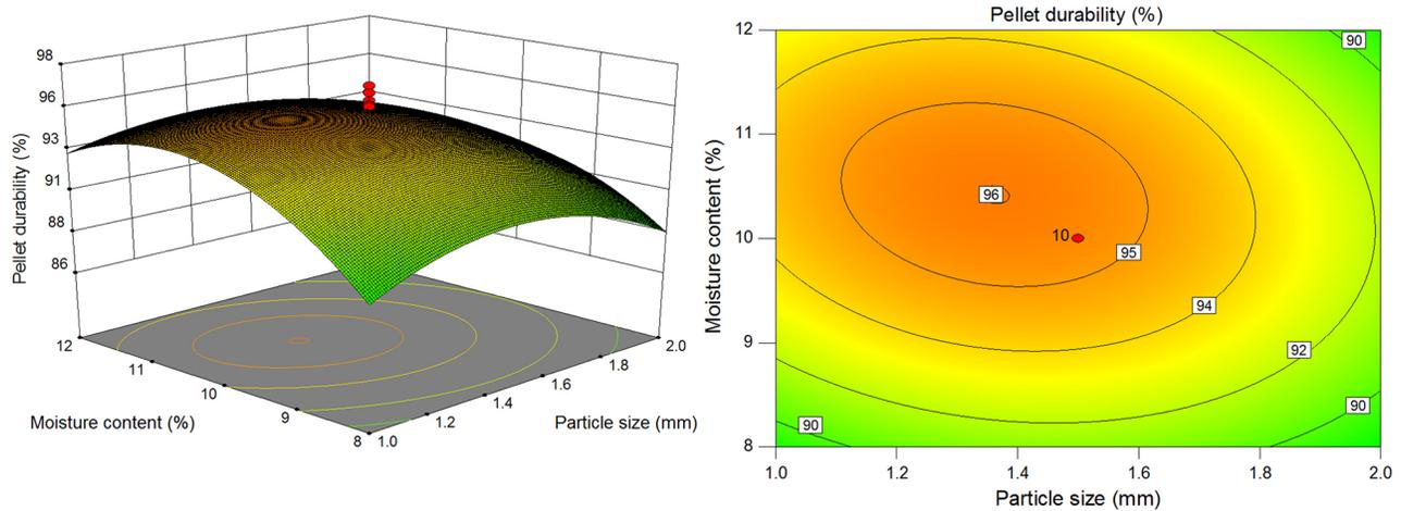
Figure 9 – Response surface of particle size and moisture content on pellet durability.
