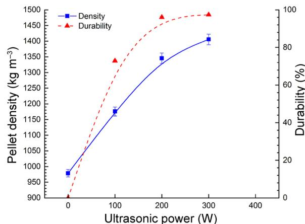
Figure 6 – Pellet density and durability with different ultrasonic powers.
