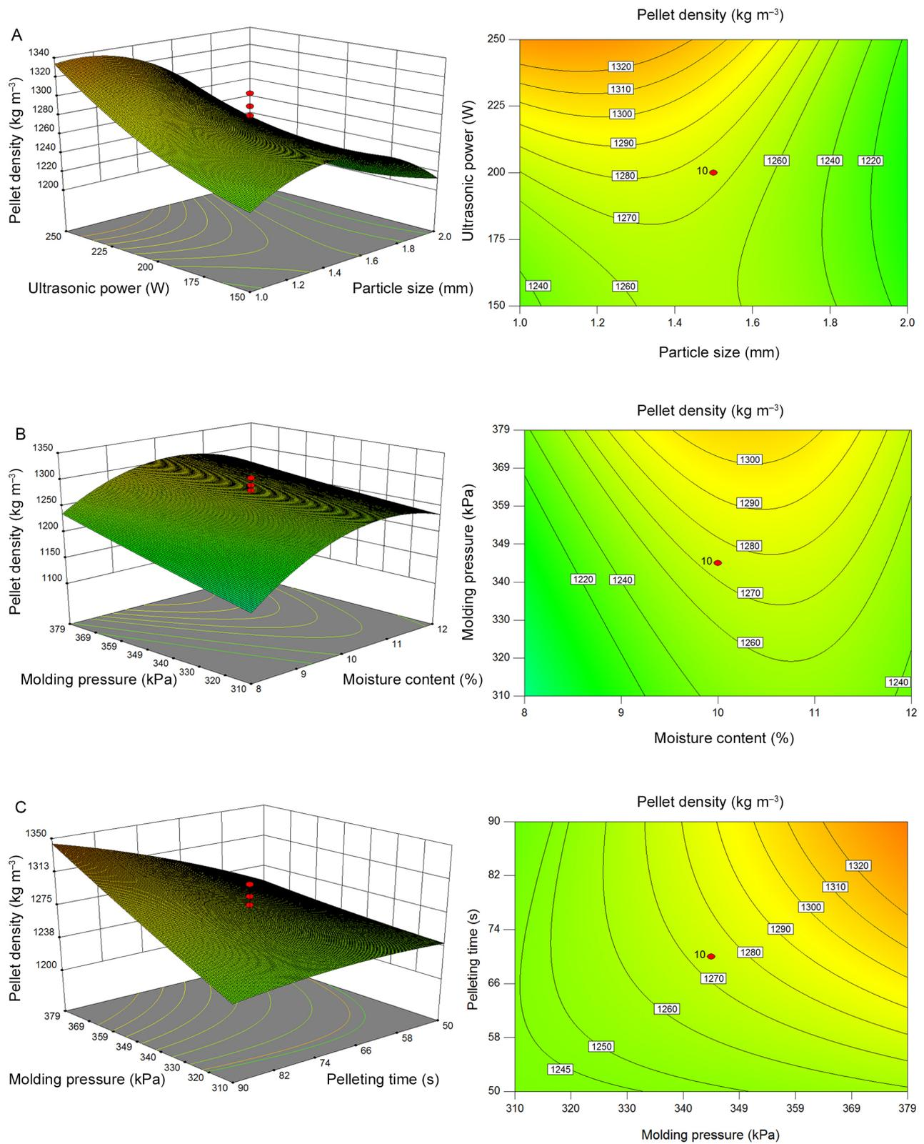
**Figure 8** – Response surface plots of pellet density between variables. (A) Particle size and ultrasonic power; (B) Moisture content and molding pressure; (C) Molding pressure and pelleting time.
