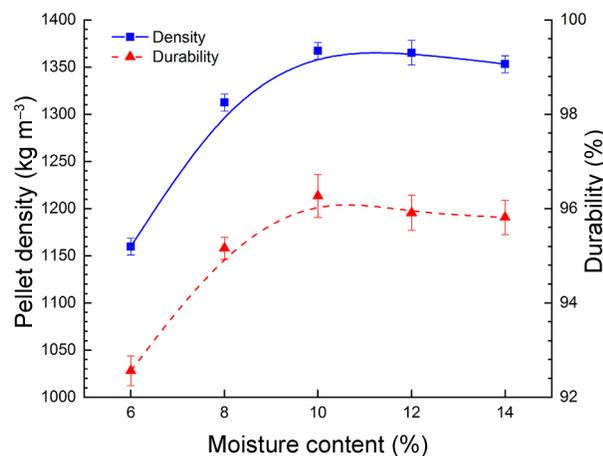
Figure 4 – Pellet density and durability with different moisture contents.
