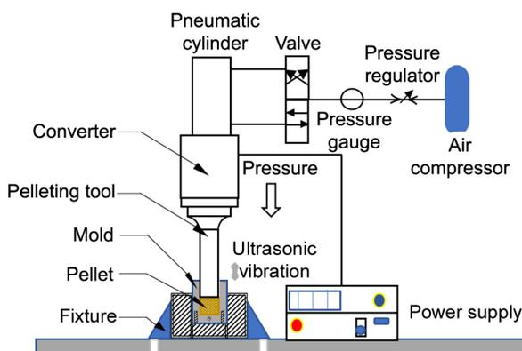
**Figure 1** – Ultrasonic assisted molding device.
