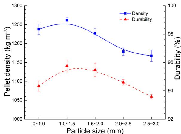
Figure 2 – Pellet density and durability with different particle sizes.
