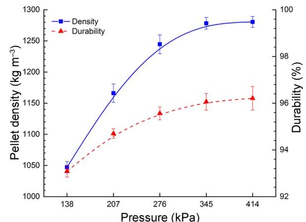
Figure 3 – Pellet density and durability with different molding pressures.
